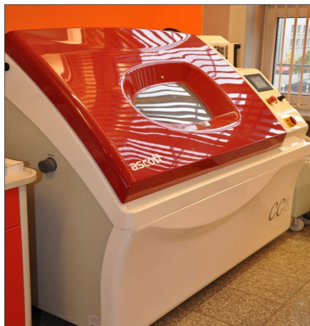
Fig. 2. Chamber (CCP450ip) used in cyclic corrosion tests in the laboratory of the Faculty of Mechanical Engineering of the Silesian University of Technology in Gliwice
