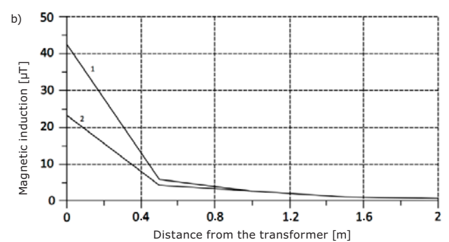
Fig. 4. Induction on the envelopes around the 800 kVA transformer: a) in the no-load state and b) in the short-circuit state
