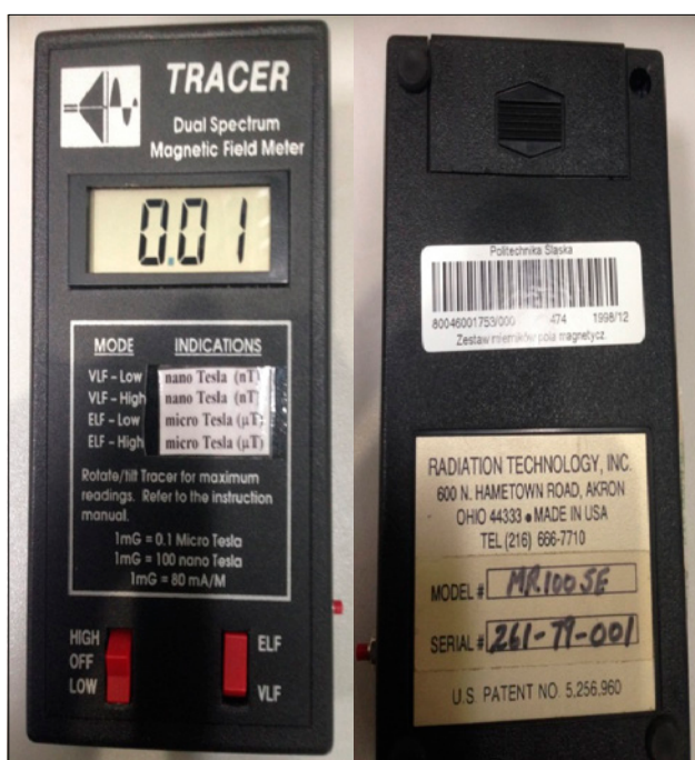
Fig. 1. Magnetic induction meter: a) obverse and b) reverse
