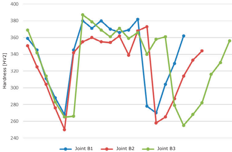
Fig. 7. Hardness distribution in the test joints
