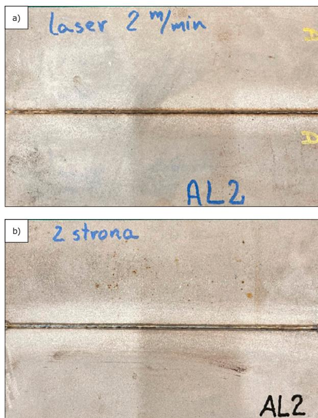
**Fig. 2.** Main view of the flat butt joint made of duplex steel LDX 2101 using a welding rate of 2 m/min: a) weld face side and b) weld root side
