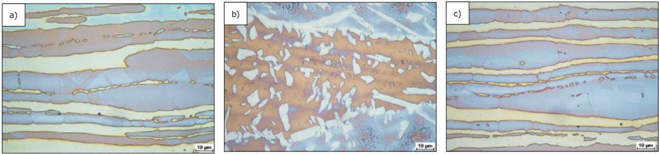
**Fig. 5.** Flat butt laser beam welded joint made of duplex steel LDX 2101 using a welding rate of 1 m/min; electrolytic etching; mag. 1000×: a) base material: brown and blue austenite, greenish and yellow ferrite, visible strain twins, b) weld and c) heat affected zone (HAZ)
