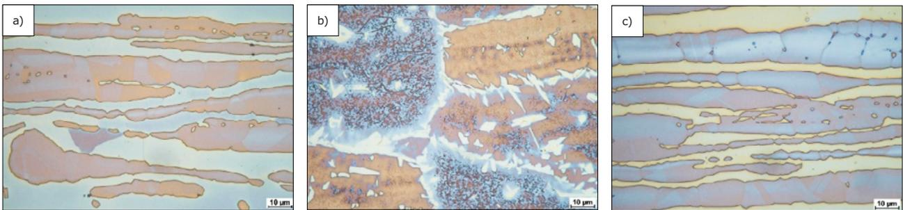
**Fig. 6.** Flat butt laser beam welded joint made of duplex steel LDX 2101 using a welding rate of 2 m/min; electrolytic etching; | mag. 1000×: a) base material: austenite with visible strain twins, greenish and yellow ferrite, b) weld and c) heat affected zone (HAZ)
