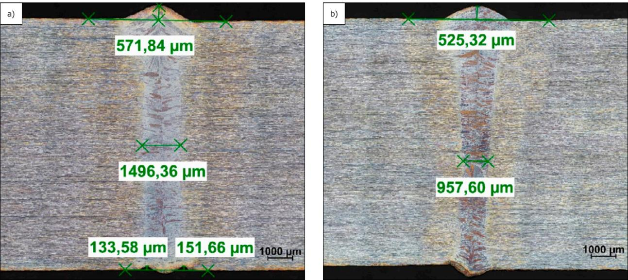
**Fig. 10.** Flat butt laser beam welded joints made of duplex steel LDX 2101, mag. 50×: a) welding rate: 1 m/min, measurements of the excess weld face metal, undercut depth on the weld root side and weld width, b) welding rate: 2 m/min, measurements of the excess weld face metal and weld width
