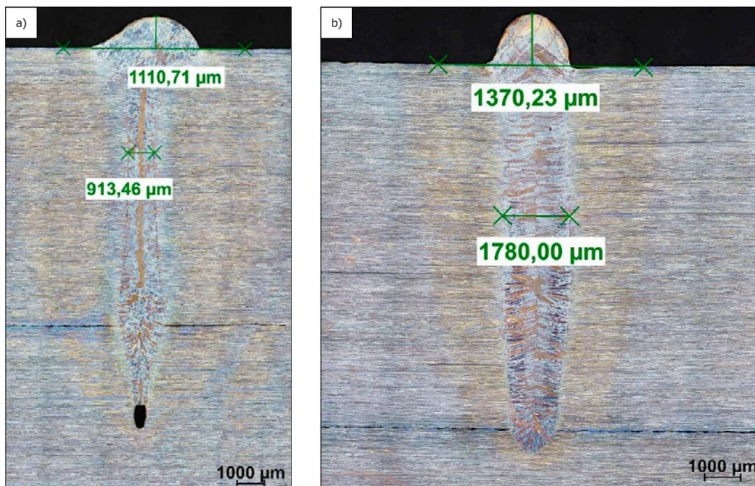
**Fig. 11.** Flat butt electron beam welded joints made of duplex steel LDX 2101, mag. 50×: a) welding rate: 0.2 m/min, measurements of the excess weld face metal and weld width and b) welding rate: 2 m/min, measurements of the excess weld face metal and weld width
