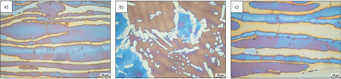
**Fig. 8.** Flat butt electron beam welded joint made of duplex steel LDX 2101 using a welding rate of 0.2 m/min; electrolytic etching; mag. 1000×: a) base material: austenite with visible strain twins, greenish and yellow ferrite, b) weld and c) heat affected zone (HAZ), strain twins visible in visible
