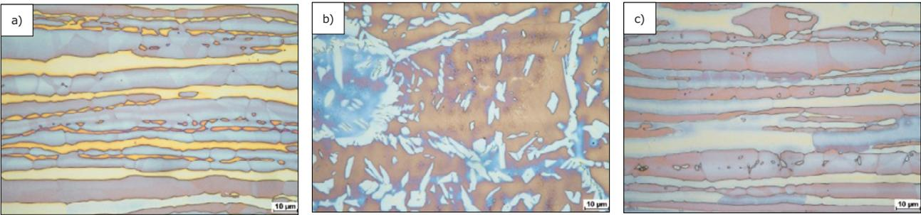
**Fig. 9.** Flat butt electron beam welded joint made of duplex steel LDX 2101 using a welding rate of 2 m/min; electrolytic etching; mag. 1000×: a) base material: austenite with visible strain twins, greenish and yellow ferrite, b) weld and c) heat affected zone (HAZ)
