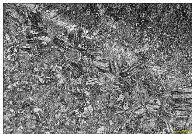
Fig. 1. Microstructure of the joint made of steel DOCOL 1300 M: a) specimen Y8 (Table 5)
