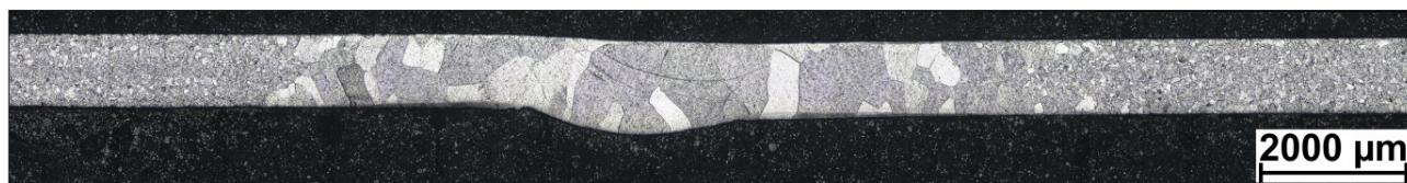
Fig. 16. Macrostructure of the girth butt welded joint - zone A
