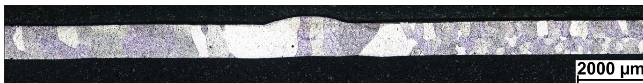
Fig. 17. Macrostructure of the girth butt welded joint - zone B
