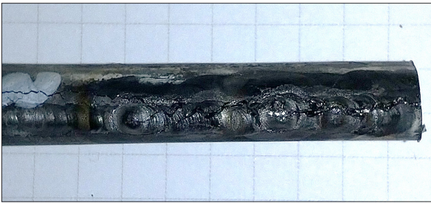
Fig. 9. Crack in the HAZ and in the weld of test joint 3A, in accordance with Fig. 7
