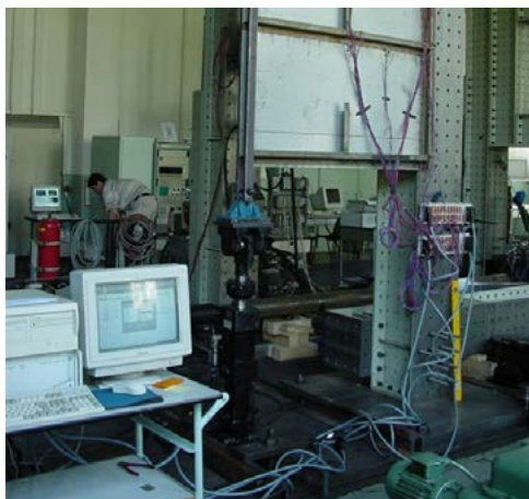
Fig. 2. Station for extensometric measurements of the side wall segment
