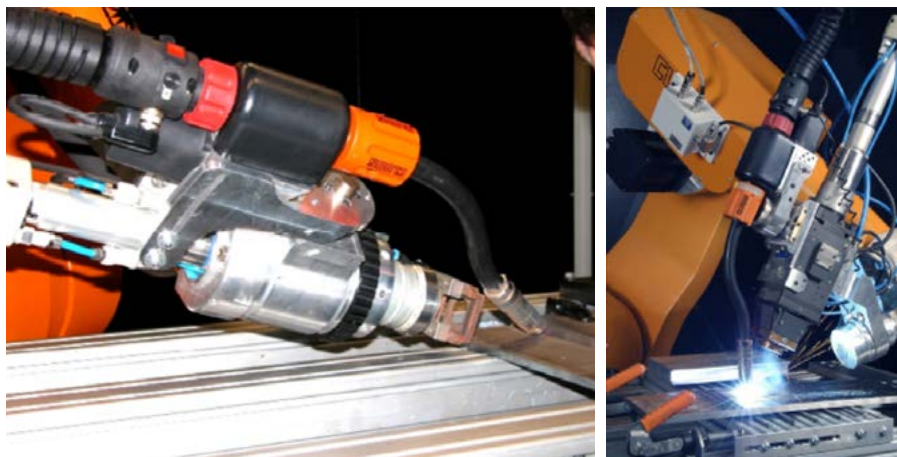
Fig. 3. Positioning for making the filler weld in the overlap joint and the head for hybrid welding with integrated welding process control sensors
