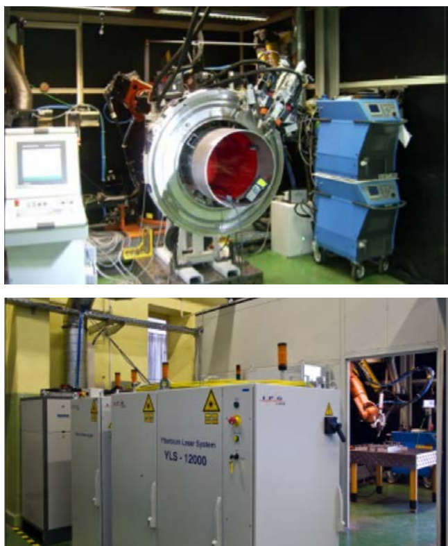
Fig. 8. Specialised prototype of a device equipped with the YLS-12000 fibre laser
