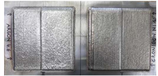
Fig. 8. CMT welded samples
