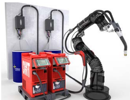
Fig. 4. Configuration CMT Twin
