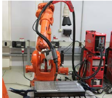
Fig. 7. Weld setup CMT Welding
