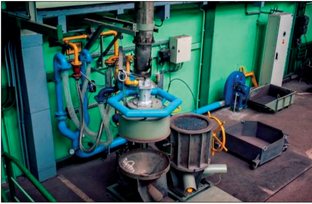
Fig. 6. Semi-industrial installation for the sintering of iron ores (left) equipped with a gas purifying system (right)
