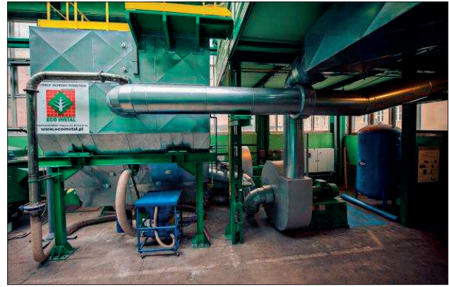
Fig. 6. Semi-industrial installation for the sintering of iron ores (left) equipped with a gas purifying system (right)
