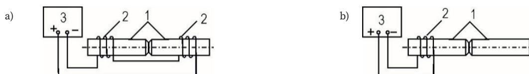
Fig. 7. Schematic diagrams of systems for eliminating residual magnetism in long elements made of steel: a) using two inductors and b) using one inductor (1 – tubular elements, 2 – magnetic inductors and 3 – power source)
