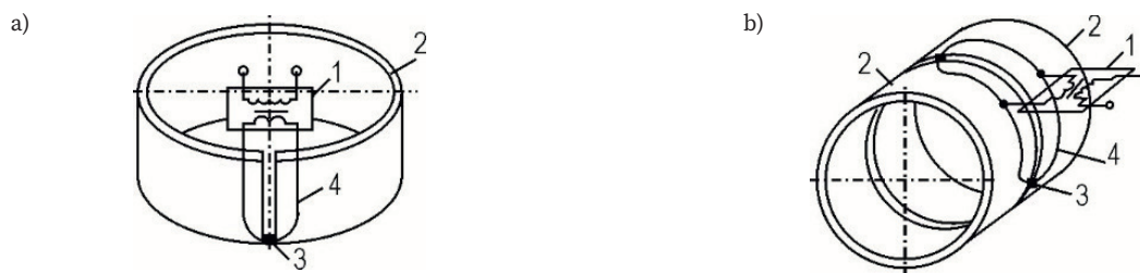
Fig. 6. Schematic diagrams of systems for eliminating the magnetic blowout effect during the welding of tubular elements (1 – single-phase transformer, 2 – steel tube, 3 – jumper and 4 – current flow circuit) [7]
