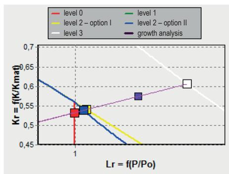
**Fig. 4.** Fragment of the FAD diagram used in the assessment of the strength of the pipe containing the internal transverse surface fracture (in accordance with the FITNET procedures); the assessment was performed using the FITNET.exe application (the purple point on the diagram corresponds to coordinates ( $L_r$  and  $K_r$ )) (own elaboration based on [1, 2, 4, 5 and 12])
