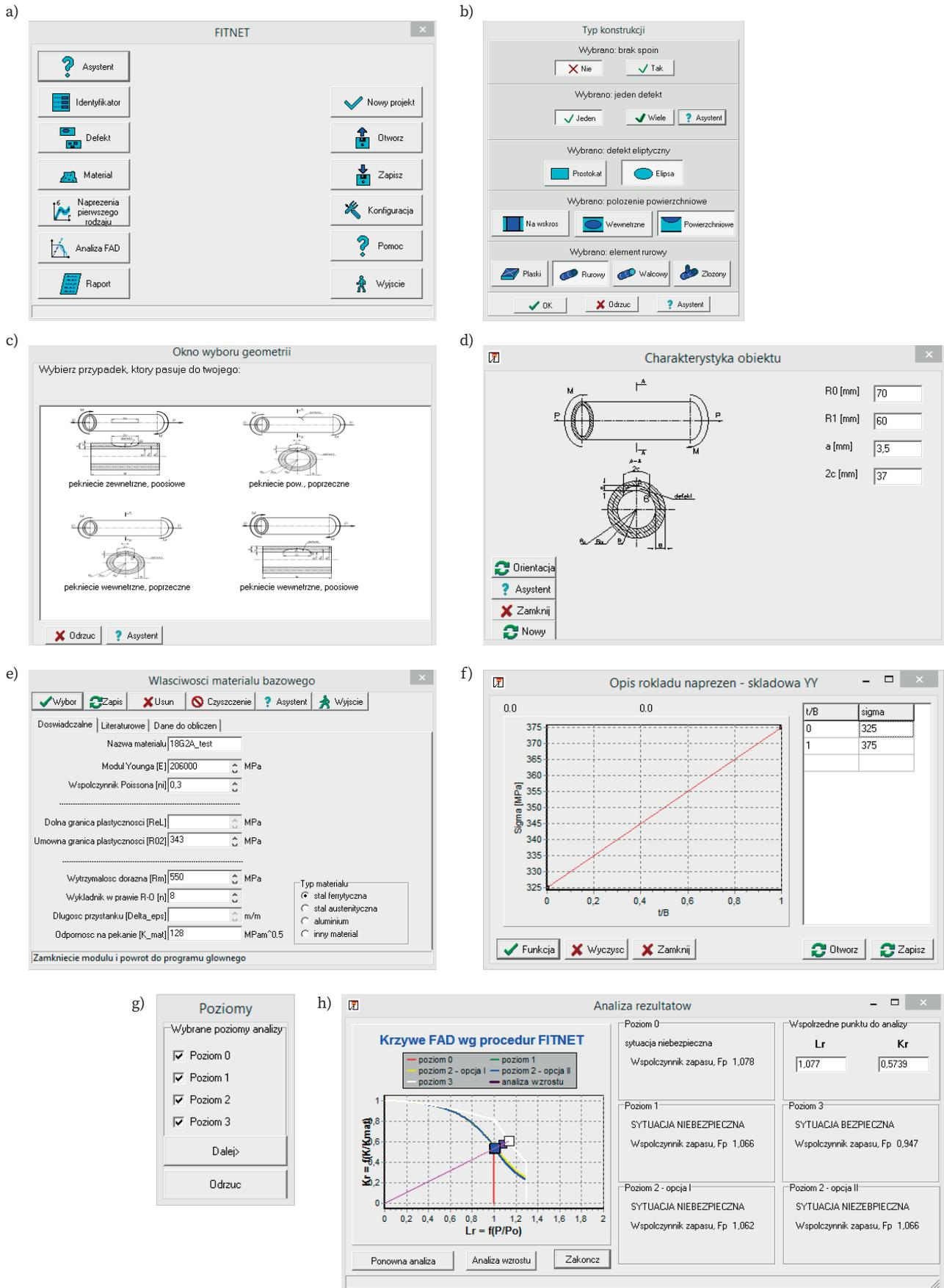
**Fig. 3.** Subsequent stages of the assessment of the strength of the pipe containing an internal transverse surface fracture in accordance with the FITNET procedures; the assessment was performed using the FITNET.exe programme (own elaboration based on [1, 2, 4, 5 and 12])
