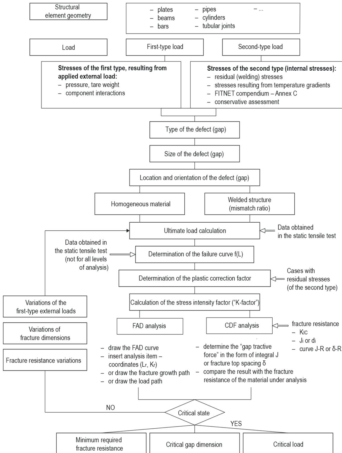
**Fig. 1.** General schematic diagram of the fracture mechanics module in the FITNET procedures (own elaboration based on [12])
