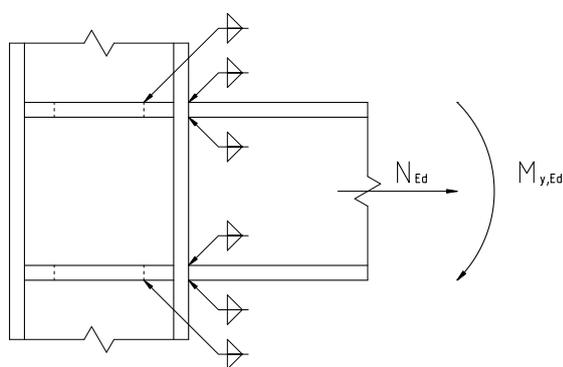
**Fig. 5.** Schematic diagram of the node with resultant loads
