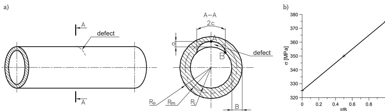
Fig. 2. Schematic diagram of a pipe containing an internal transverse surface fracture (own elaboration based on [2, 4, 5, 12])
