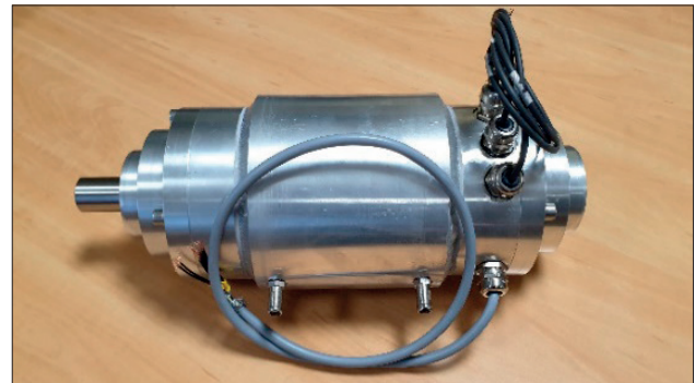
Fig. 1. High-speed generator PMzK71-4 having a power of 17 kW, fabricated by Łukasiewicz – GIT
