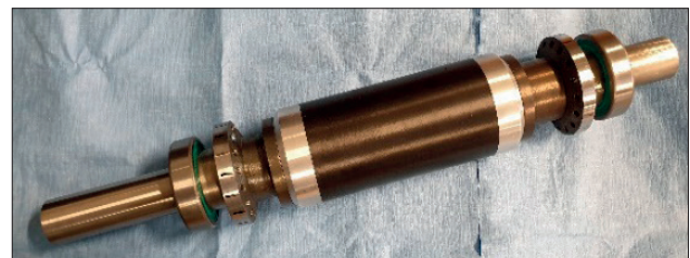
Fig. 2. Rotor of the PMzK71-4 generator with CFRP composite sleeve and hybrid bearings
