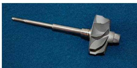
Fig. 8. Electron beam welding of supercharger shafts a) device, b) element after welding [18]
