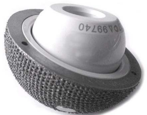
Fig. 14. Example of the electron beam use for fast prototyping of endoprosthesis elements [22]
