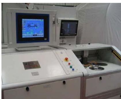
Fig. 7. Electron beam welding of toothed gear elements [19]
