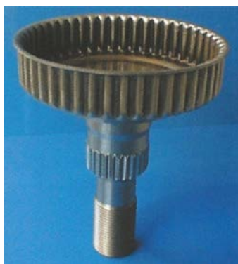
Fig. 7. Electron beam welding of toothed gear elements [19]
