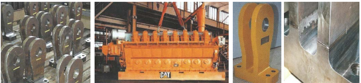
Fig. 11. Electron beam welding of transport hooks made of high-strength steel [19]
