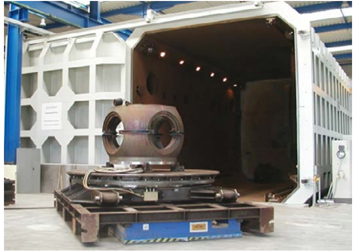
Fig. 10. Electron beam welding of a wind tower element – rotor cap [21]
