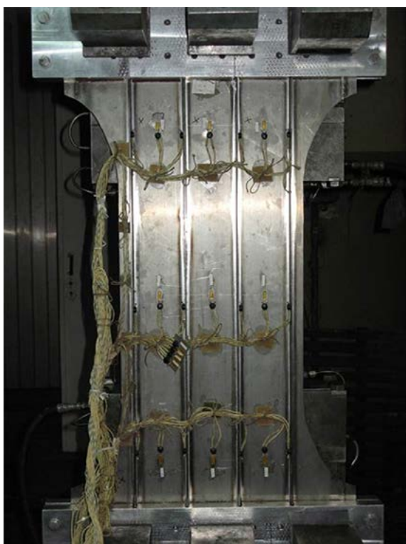
Fig. 8. Panel with strain gauges fixed in the clamps of the fatigue testing machine
