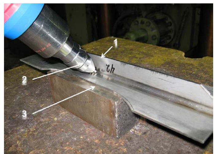
Fig. 6. Treatment with the manual impact testing machine using HFPMT of the T-joint made of the VT-20 alloy; 1- specimen subjected to treatment; 2- impact testing machine head; 3-plate.
