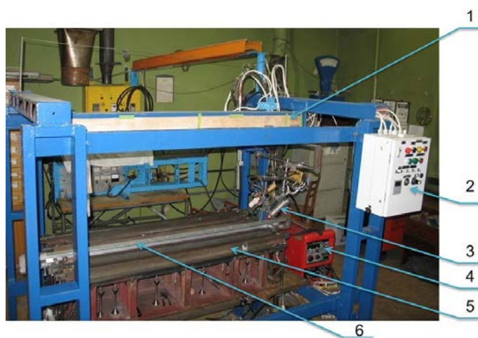
Fig. 3. Laboratory stand for TIG welding of ribbed panels in preliminary deforming conditions: 1 – gantry with the welding head travel car; 2 – control system; 3 – welding head; 4 – power source; 5 – loading system for preliminary elastic deforming of elements welded; 6 – welded panel
