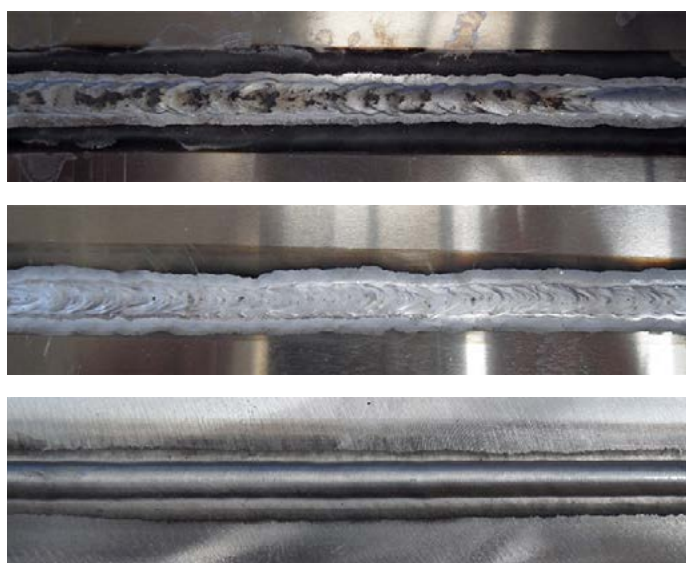
Fig. 1. View of the welded joint made of the 2.0 mm thick EN AW 7075 alloy, a) - b) MIG-Pulse, c) CMT
