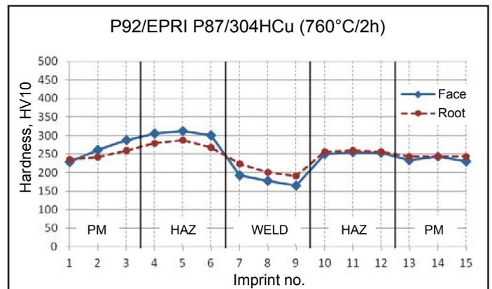
Fig. 16. Hardness of butt joint of the P92 and 304HCu steel pipes welded with the EPRI P87 filler metal wire in the as welded state and after HT 760°C/2h
