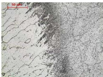
Fig. 7. Fusion line between the P92 steel and the Thermanit 304HCu weld after heat treatment 760°C/24h; the visible zone of carbon diffusion from the steel to the weld
