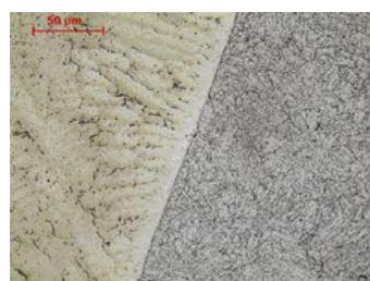
Fig. 11. Fusion line between the P92 steel and the EPRI P87 weld after heat treatment 760°C/8h; no traces of carbon diffusion
