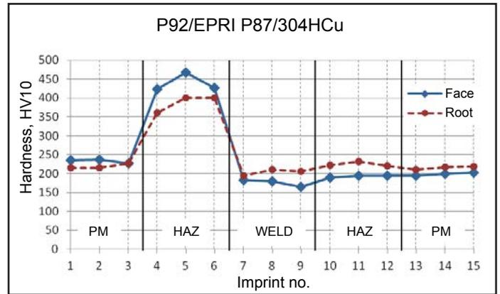
Fig. 14. Hardness of butt joint of the P92 and 304HCu steel pipes welded with the EPRI P87 filler metal wire in the as welded state
