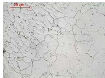
Fig. 6. Fusion line between the 304HCu steel and the EPRI P87 weld; the visible presence of epitaxial crystallisation
