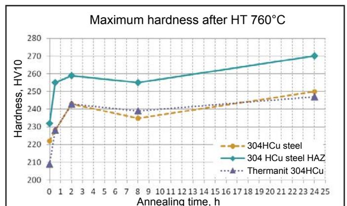
Fig. 18. Change of the maximum hardness values of the 304HCu steel, the 304HCu steel HAZ and of the weld made using the 304HCu filler metal in the function of heat treatment time at 760°C
