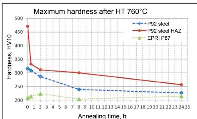
Fig. 17. Change of the maximum hardness values of the P92 steel, the P92 steel HAZ and of the weld made using the EPRI P87 filler metal in the function of heat treatment time at 760°C
