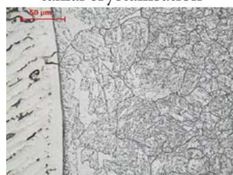
Fig. 9. Fusion line between the P92 steel and the Thermanit 304HCu weld after heat treatment 760°C/8h; the visible presence of ferrite  $\delta$  in the HAZ coarse-grained area
