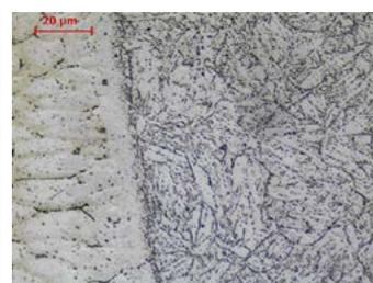
Fig. 12. Fusion line between the P92 steel and the EPRI P87 weld after heat treatment 760°C/24h; no traces of carbon diffusion
