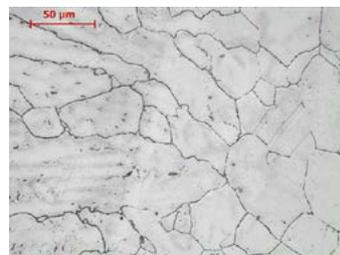
Fig. 5. Fusion line between the 304HCu steel and the Thermanit 304HCu weld; the visible presence of epitaxial crystallisation
