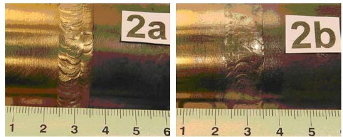
Fig. 1. Weld face view of the joint made of the P92 and 304HCu steels welded with the Thermanit 304HCu (2a) and EPRI P87 (2b) wires
