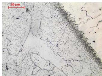
Fig. 8. Fusion line between the P92 steel and the Thermanit 304HCu weld after heat treatment 760°C/2h; the visible zone of carbon diffusion from the steel to the weld and the presence of ferrite  $\delta$  in the HAZ coarse-grained area
