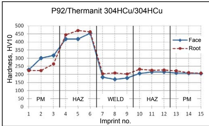
Fig. 13. Hardness of butt joint of the P92 and 304HCu steel pipes welded with the Thermanit 304HCu filler metal wire in the as welded state
