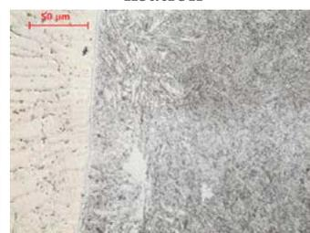
Fig. 10. Fusion line between the P92 steel and the EPRI P87 weld; the visible presence of ferrite  $\delta$  in the HAZ coarse-grained area
