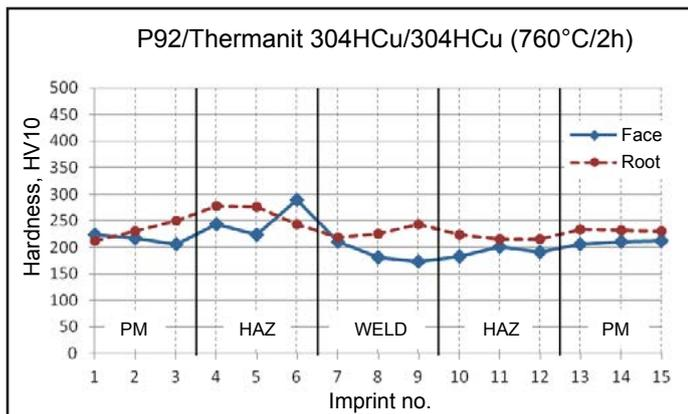
Fig. 15. Hardness of butt joint of the P92 and 304HCu steel pipes welded with the Thermanit 304HCu filler metal wire in the as welded state and after HT 760°C/2h
