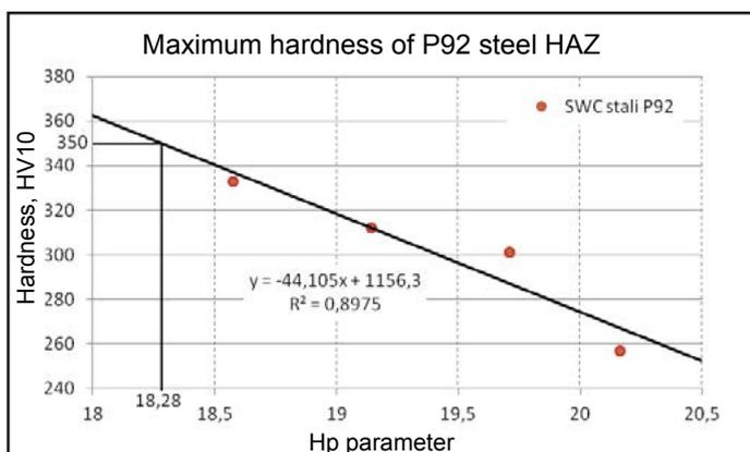
Fig. 19. Maximum hardness of the P92 steel HAZ depending on the  $Hp$  parameter
