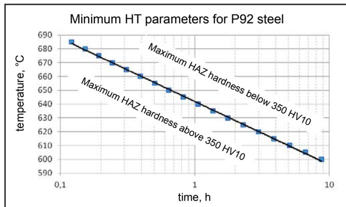
Fig. 20. Correlation between the annealing temperature and the hold time determined on the basis of the Hollomon-Jaffe dependence for the P92 steel HAZ
