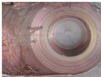
Fig. 3. Weld face after the welding process. Welding parameters: V_n = 450 rev/min, V_z = 71 mm/min. Conical tool S(1). Process conducted with the tool inclination angle of 1.5^\circ
