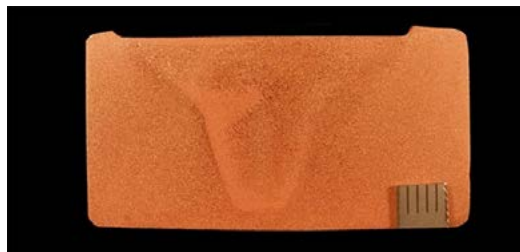
Fig. 7. Structure of FSW plasticised material (copper). Tool S(5). Welding parameters: V_n = 450 rev/min, V_z = 71 mm/min
