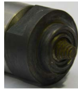
Fig. 2. Tool working part used in the FSW and FSP tests
