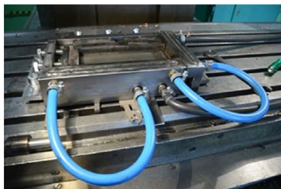
Fig. 6. Welding device provided with the welding area cooling system installed on the FY 40 milling machine
