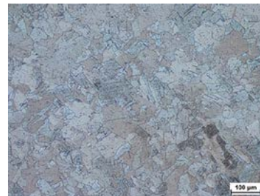
Fig. 19. Recrystallised structure of the central FSW weld area from the retreat side; etching with FeCl 3
