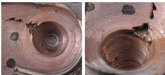
Fig. 5. Weld face view at the weld end area after the welding process. Welding parameters: V_n = 355 rev/min, V_z = 71 mm/min. Conical tool S(3). Process conducted without the tool inclination angle
