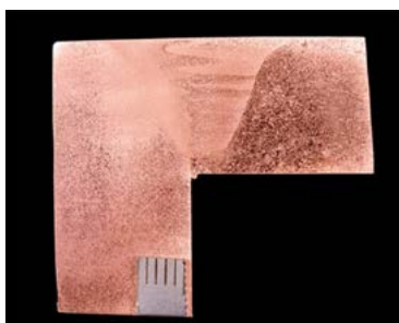
Fig. 16. Macrostructure of the joint made of copper plates using the technology developed. V_n = 560 \text{ rev/min} ; V_z = 71 \text{ mm/min}
