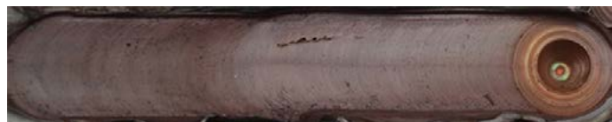
Fig. 4. Weld face after the welding process. Welding parameters: V_n = 355 rev/min, V_z = 71 mm/min. Conical tool S(3). Process conducted without the tool inclination angle
