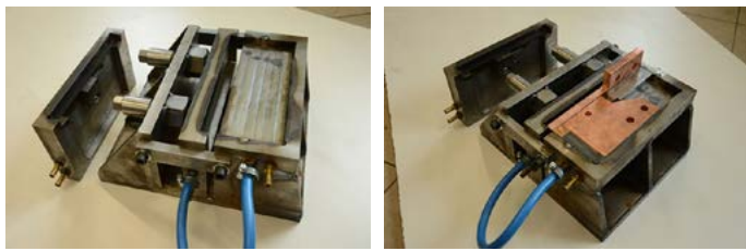
Fig. 13. Tooling for fixing the conductor rails: a) view without welding elements, b) view with welding rails. On the left: the exchangeable pressure plate
