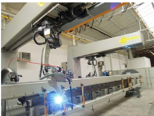
Fig. 8. Stand for welding lorry semitrailer elements; the tight field for welding stringers
