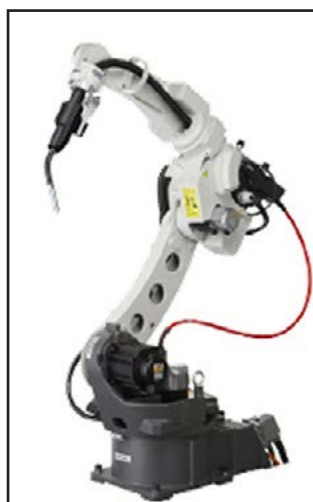
Fig. 6. TM robot with the conduits guided inside the arm
