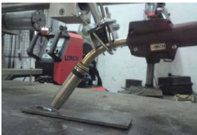
Fig. 2. Welding test rig featuring the progressive manipulator during recording current waveforms in time
