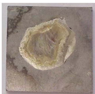
Fig. 4. Wettability of the Ag 245 filler metal on the X2CrNi18-9 grade stainless steel using the F10 flux
