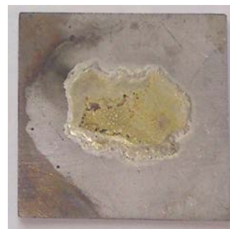
Fig. 2. Spreadability of the Ag 245 filler metal on the X2CrNi18-9 grade stainless steel using the F6B flux
