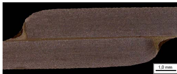
Fig. 1. Macrostructure of the joint made of the X2CrNi18 stainless steel, brazed with the Ag 145 grade coated silver filler metal, etchant: \text{FeCl}_2
