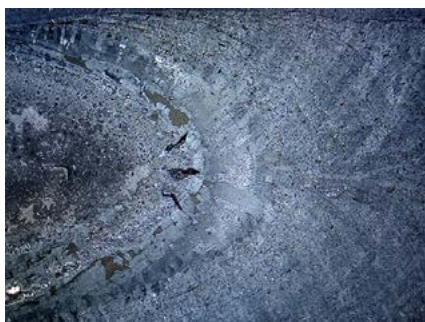
Fig. 3. 5 mm thick 304 (155) steel, bend radius of 135 mm. Fusion face. Cracks in the L+S zone. The longest crack of 1 mm, LM, mag. 10x,
