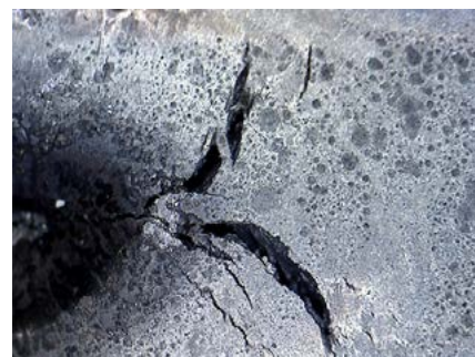
Fig. 4. 3 mm thick 314 (335) steel, bend radius of 135 mm. Fusion face. Cracks in the L+S zone. The longest crack of 2 mm, LM, mag. 10x
