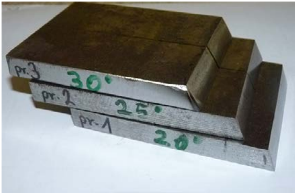
Fig. 2. Specimens for tests no. 1, 2 and 3 beveling angles \beta = 20^\circ, 25^\circ and 30^\circ
