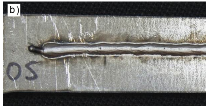
Fig. 3. Commencement of laser melting with a filler metal with excessive exposed length of the wire recorded with a fast camera (a); the view of the face of a fusion bead with a wire end welded onto the beginning of the bead (b)
