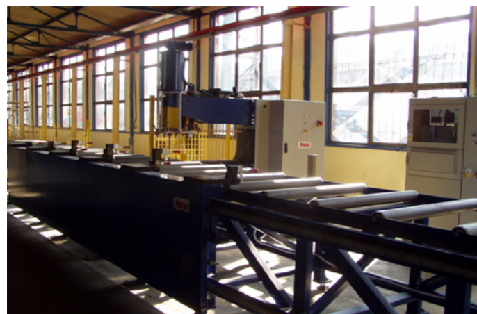
Fig. 2. Station for welding car body components produced by the ASPA company
