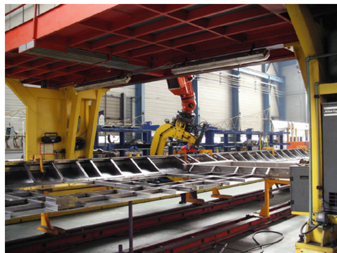
Fig. 3. Station for welding car body components – the Bisiach & Carru company gantry
