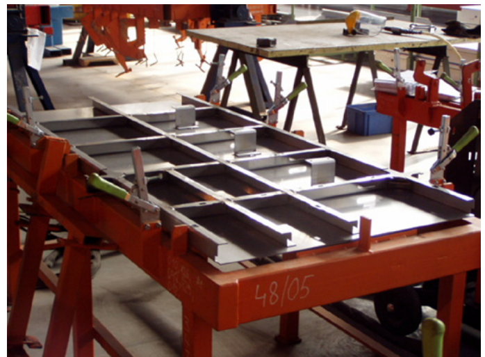
Fig. 6. Station for car body component assembly
