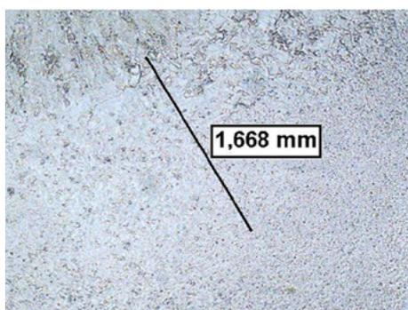
Fig. 4. Microstructure and HAZ width measurement result for the minimum EN ratio setting. Magnification x25. Etchant: Nital
