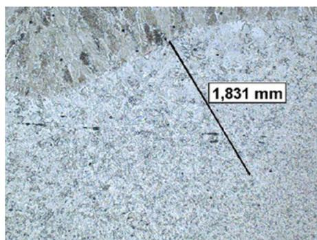
Fig. 3. Microstructure and HAZ width measurement result for the neutral EN ratio setting. Magnification x25. Etchant: Nital
