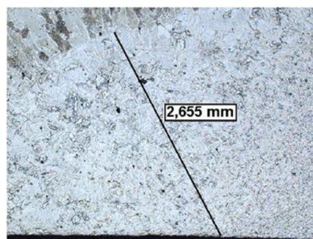
Fig. 5. Microstructure and HAZ width measurement result for the maximum EN ratio setting. Magnification x25. Etchant: Nital
