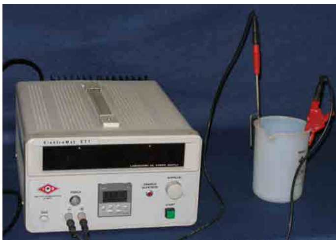
Fig. 3. Device for electrolytic etching ElektroMat ET1
