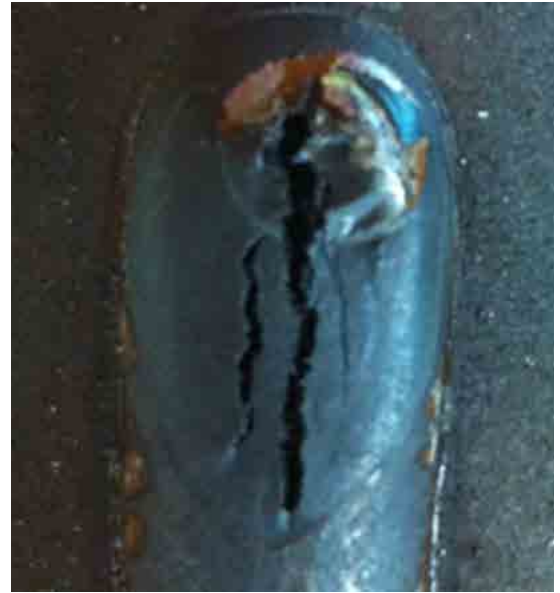
Fig. 3. Solidification crack in the crater of weld made on 12mm-thick plate with 20% strain, used in Transvarestraint test
