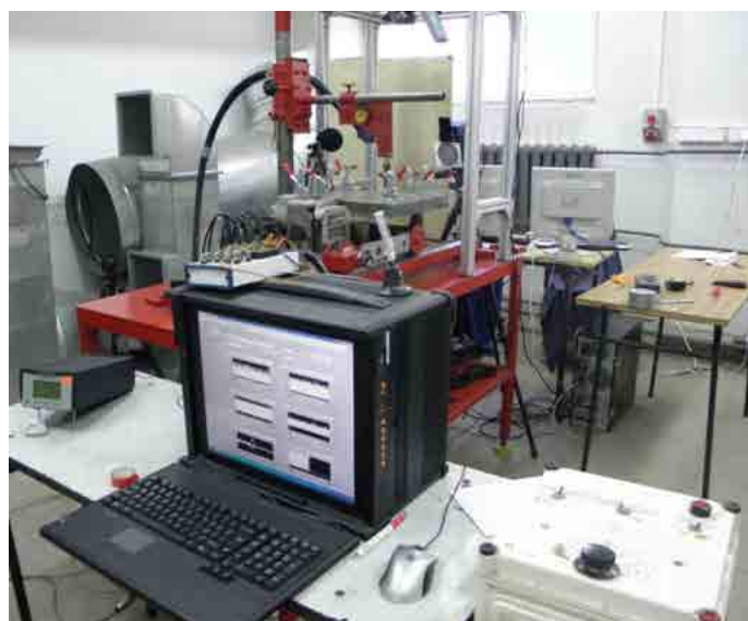
Fig. 2. Mechanised station for MAG welding
