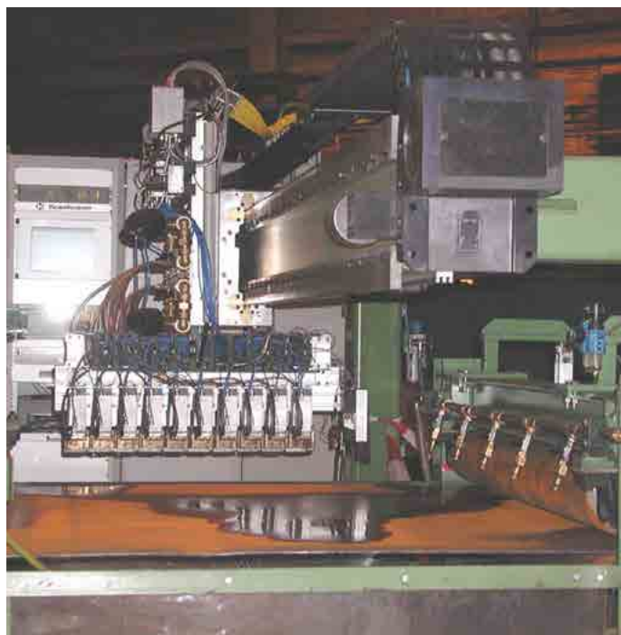
Fig. 2. Device applied in UT of strips for the presence of laminar imperfections, used in the Salzgitter Mannesmann Grossrohr GmbH company, Germany [5]
