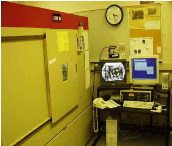
Fig. 6. Example of device for radiosopic testing of welded joints
