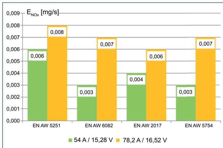
Fig. 20 NO<sub>x</sub> emission while welding aluminium alloys of 5xxx, 6xxx and 2xxx series with AC Pulse method using filler metal grade AlMg4.5MnZr φ1.2 mm, in Ar-based shielding gas
