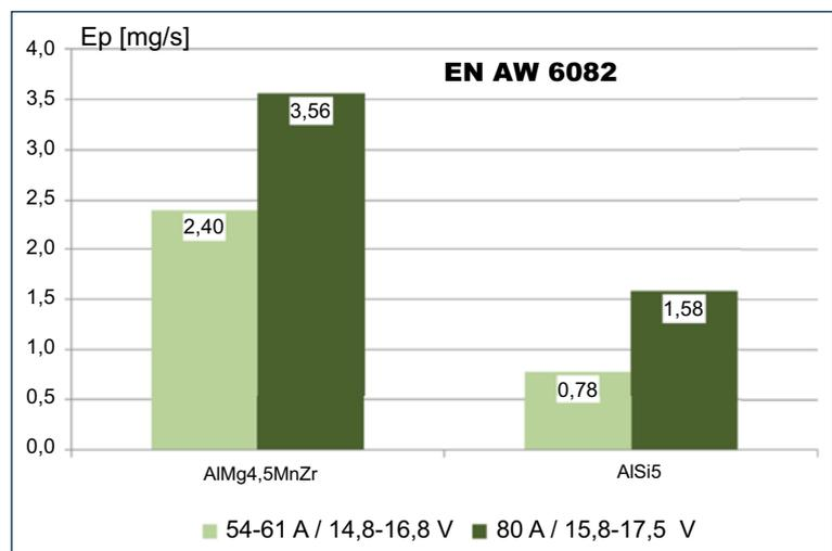
Fig. 4 Dust emission while welding aluminium alloy EN AW 6082 with Cold Process method using filler metal grades AlMg4.5MnZr and AlSi5r  $\phi$ 1.2 mm, in Ar-based shielding gas
