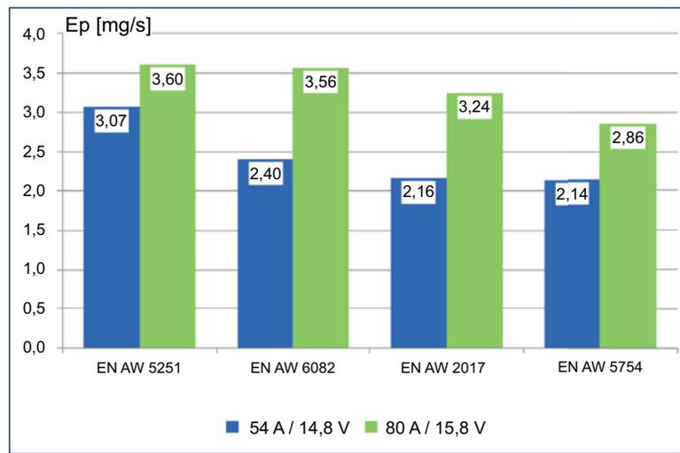
Fig. 3 Dust emission while welding aluminium alloys of 5xxx, 6xxx and 2xxx series with Cold Process method using filler metal grade AlMg4.5MnZr  $\phi$ 1.2 mm, in Ar-based shielding gas
