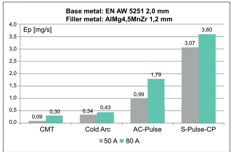
Fig. 28 Dust emission while welding alloy EN AW 5251 with CMT, ColdArc , Cold Process (S-Pulse-CP) and AC Pulse methods and filler metal AlMg4.5MnZr
