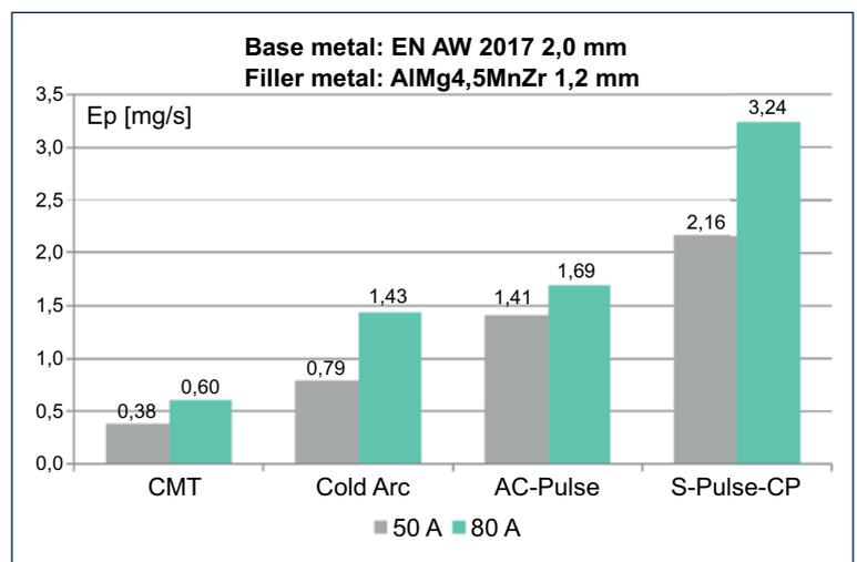
Fig. 30 Dust emission while welding alloy EN AW 1070 with CMT, ColdArc , and Cold Process (S-Pulse-CP) methods and filler metal AlMg4.5MnZr
