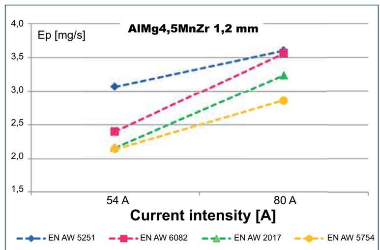
Fig. 13. Impact of current intensity on dust emission while welding aluminium alloys of 5xxx, 6xxx and 2xxx series with Cold Process method using filler metal grade AlMg4.5MnZr φ1.2 mm, in Ar-based shielding gas
