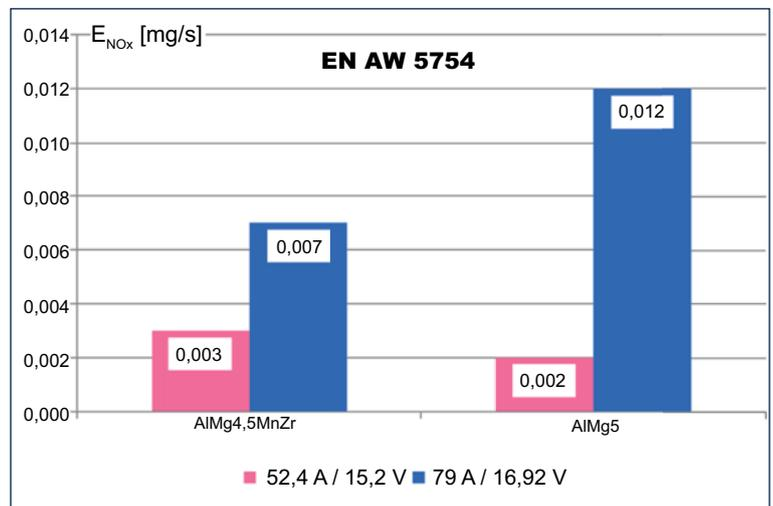
Fig. 24 NO<sub>x</sub> emission while welding aluminium alloy EN AW 5754 with AC Pulse method using filler metal grades AlMg4.5MnZr and AlMg5 φ1.2 mm, in Ar-based shielding gas
