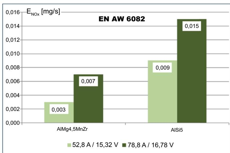
Fig. 22 NO<sub>x</sub> emission while welding aluminium alloy EN AW 6082 with AC Pulse method using filler metal grades AlMg4.5MnZr and AlSi5r φ1.2 mm, in Ar-based shielding gas
