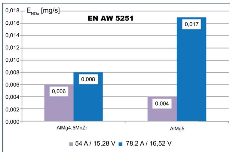
Fig. 21 NO<sub>x</sub> emission while welding aluminium alloy EN AW 5251 with AC Pulse method using filler metal grades AlMg4.5MnZr and AlMg5Cr φ1.2 mm, in Ar-based shielding gas
