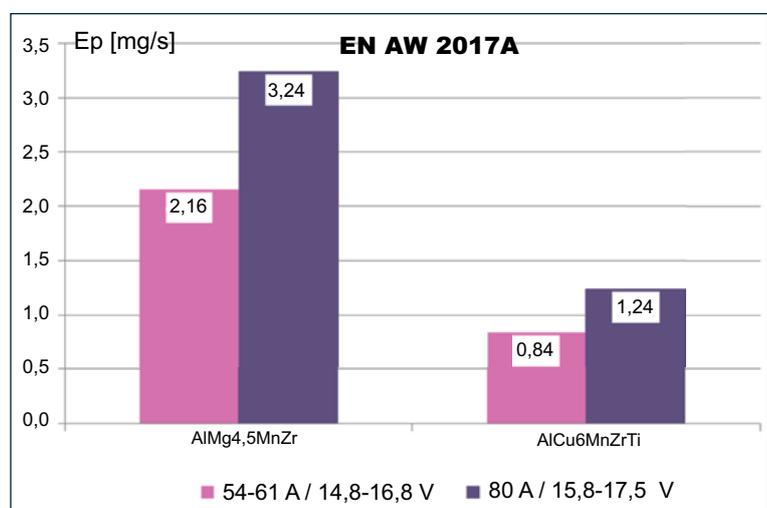
Fig. 5 Dust emission while welding aluminium alloy EN AW 2017A with Cold Process method using filler metal grades AlMg4.5MnZr and AlCu6MnZrTi  $\phi$ 1.2 mm, in Ar-based shielding gas
