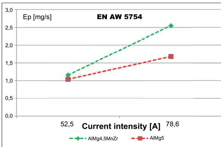
Fig. 26. Impact of current intensity on dust emission while welding aluminium alloy EN AW 5754 with AC Pulse method using filler metal grades AlMg4.5MnZr and AlMg5  $\phi$ 1.2 mm, in Ar-based shielding gas
