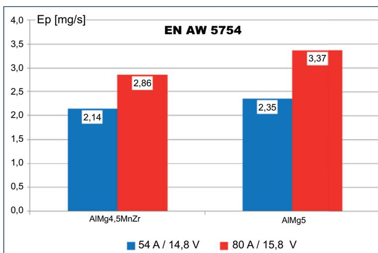
Fig. 7 Dust emission while welding aluminium alloy EN AW 5754 with Cold Process method using filler metal grades AlMg4.5MnZr and AlMg5  $\phi$ 1.2 mm, in Ar-based shielding gas
