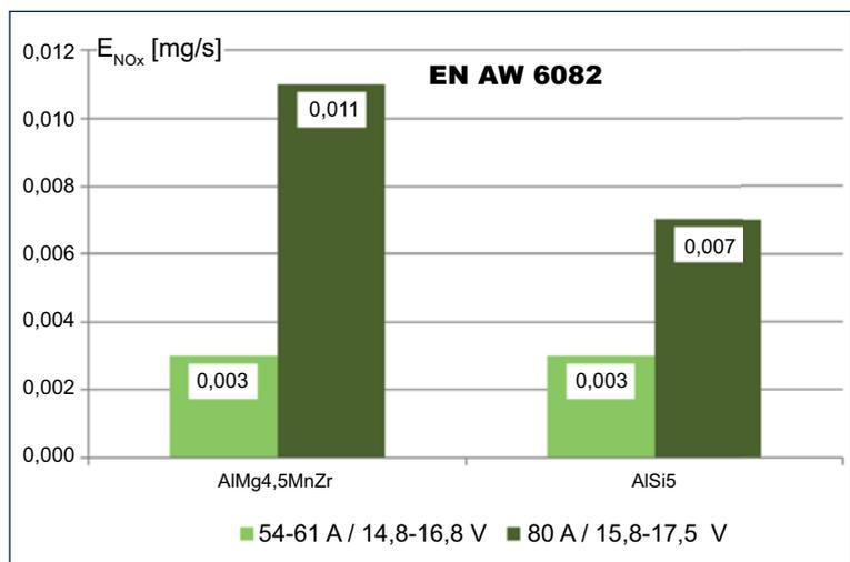
Fig. 10 NO<sub>x</sub> emission while welding aluminium alloy EN AW 6082 with Cold Process method using filler metal grades AlMg4.5MnZr and AlSi5r φ1.2 mm, in Ar-based shielding gas
