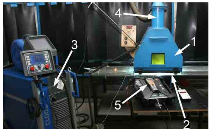
Fig. 1. Test station for testing emissions of dust and gases during welding with Cold Process method, device QINEO CHAMP 450 Cloos
