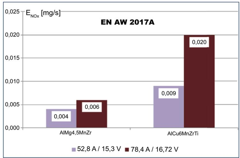
Fig. 23 NO<sub>x</sub> emission while welding aluminium alloy EN AW 2017A with AC Pulse method using filler metal grades AlMg4.5MnZr and AlCu6MnZrTi φ1.2 mm, in Ar-based shielding gas
