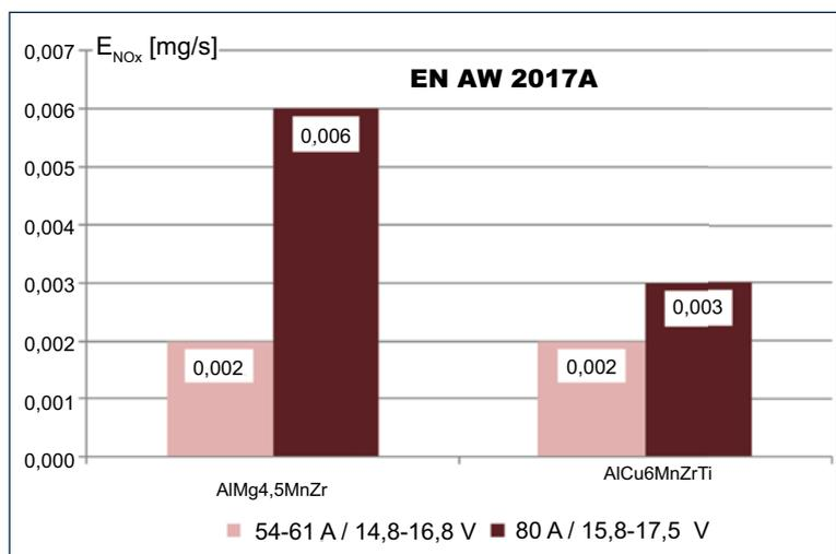
Fig. 11 NO<sub>x</sub> emission while welding aluminium alloy EN AW 2017A with Cold Process method using filler metal grades AlMg4.5MnZr and AlCu6MnZrTi φ1.2 mm, in Ar-based shielding gas
