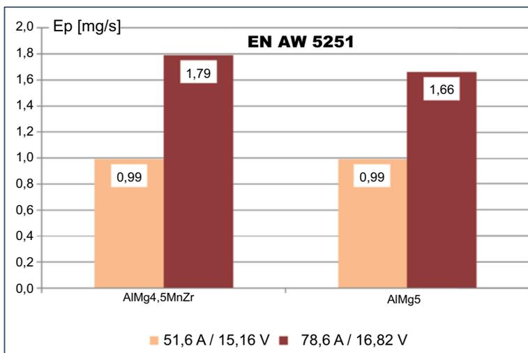
Fig. 18 Dust emission while welding aluminium alloy EN AW 5251 with AC Pulse method using filler metal grades AlMg4.5MnZr and AlMg5Cr  $\phi$ 1.2 mm, in Ar-based shielding gas
