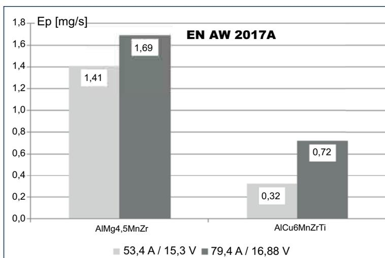
Fig. 16 Dust emission while welding aluminium alloy EN AW 2017A with AC Pulse method using filler metal grades AlMg4.5MnZr and AlCu6MnZrTi  $\phi$ 1.2 mm, in Ar-based shielding gas
