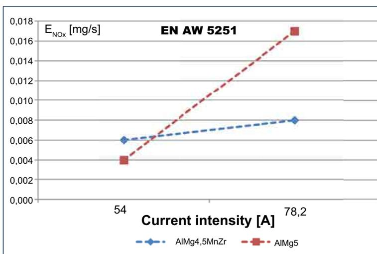
Fig. 27. Impact of current intensity NO<sub>x</sub> emission while welding aluminium alloy EN AW 5251 with AC Pulse method using filler metal grades AlMg4.5MnZr and AlMg5Cr  $\phi$ 1.2 mm, in Ar-based shielding gas
