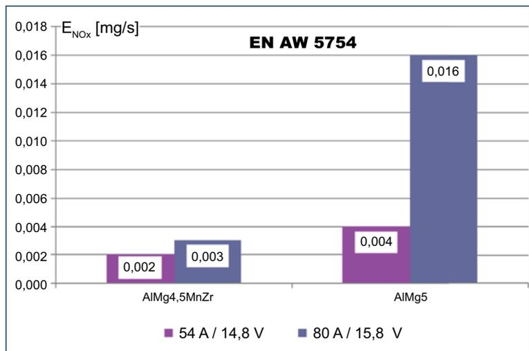
Fig. 9 NO<sub>x</sub> emission while welding aluminium alloy EN AW 5754 with Cold Process method using filler metal grades AlMg4.5MnZr and AlMg5 φ1.2 mm, in Ar-based shielding gas
