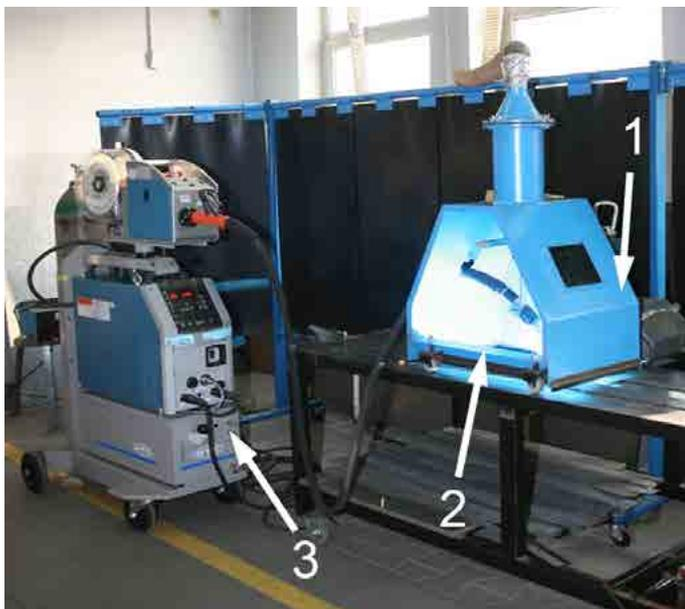
Fig. 2. Test station for testing emissions of dust and gases during welding with AC Pulse method; device DW 300 OTC Daihen.
