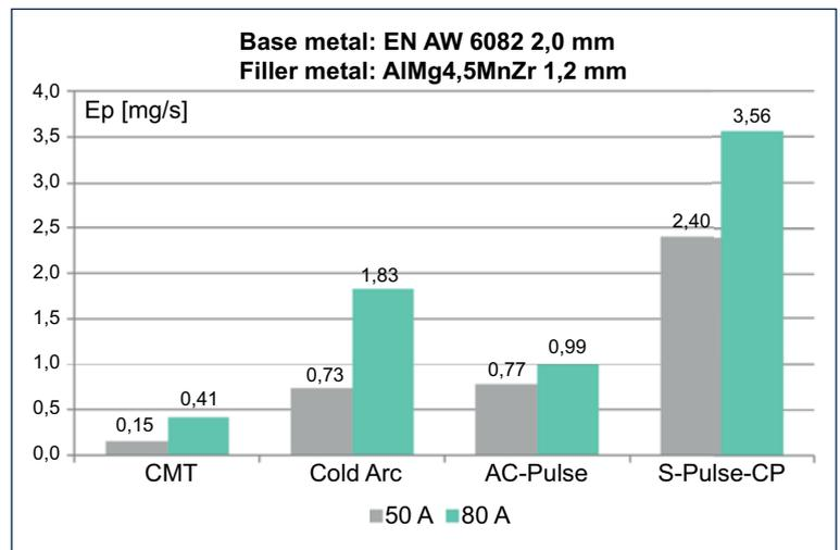
Fig. 29 Dust emission while welding alloy EN AW 6082 with CMT, ColdArc , Cold Process (S-Pulse-CP) and AC Pulse methods and filler metal AlMg4.5MnZr
