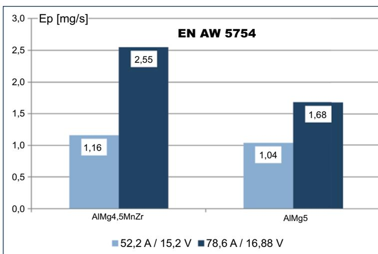
Fig. 19 Dust emission while welding aluminium alloy EN AW 5754 with AC Pulse method using filler metal grades AlMg4.5MnZr and AlMg5  $\phi$ 1.2 mm, in Ar-based shielding gas
