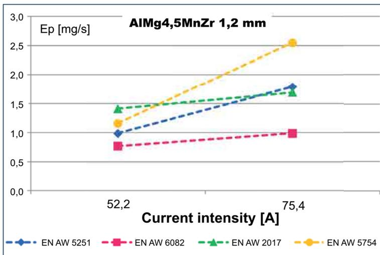
Fig. 25. Impact of current intensity on dust emission while welding aluminium alloys of 5xxx, 6xxx and 2xxx series with AC Pulse method using filler metal grade AlMg4.5MnZr  $\phi$ 1.2 mm, in Ar-based shielding gas
