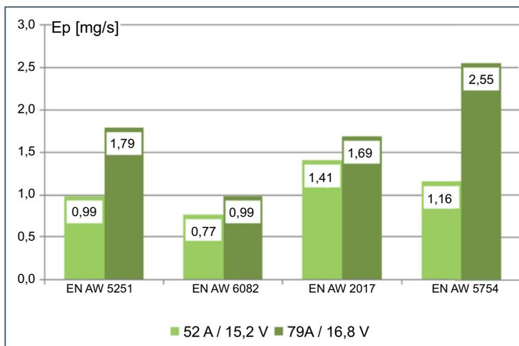
Fig. 15 Dust emission while welding aluminium alloys of 5xxx, 6xxx and 2xxx series with AC Pulse method using filler metal grade AlMg4.5MnZr  $\phi$ 1.2 mm, in Ar-based shielding gas
