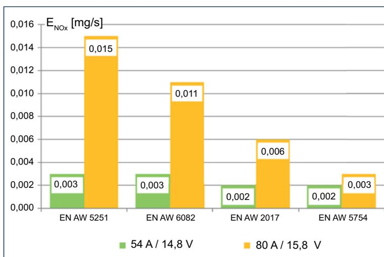
Fig. 8 NO<sub>x</sub> emission while welding aluminium alloys of 5xxx, 6xxx and 2xxx series with Cold Process method using filler metal grade AlMg4.5MnZr  $\phi$ 1.2 mm, in Ar-based shielding gas
