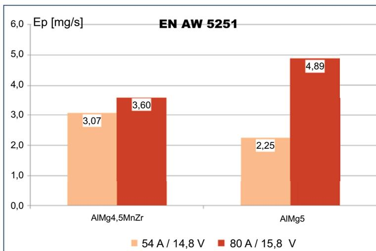
Fig. 6 Dust emission while welding aluminium alloy EN AW 5251 with Cold Process method using filler metal grades AlMg4.5MnZr and AlMg5Cr  $\phi$ 1.2 mm, in Ar-based shielding gas
