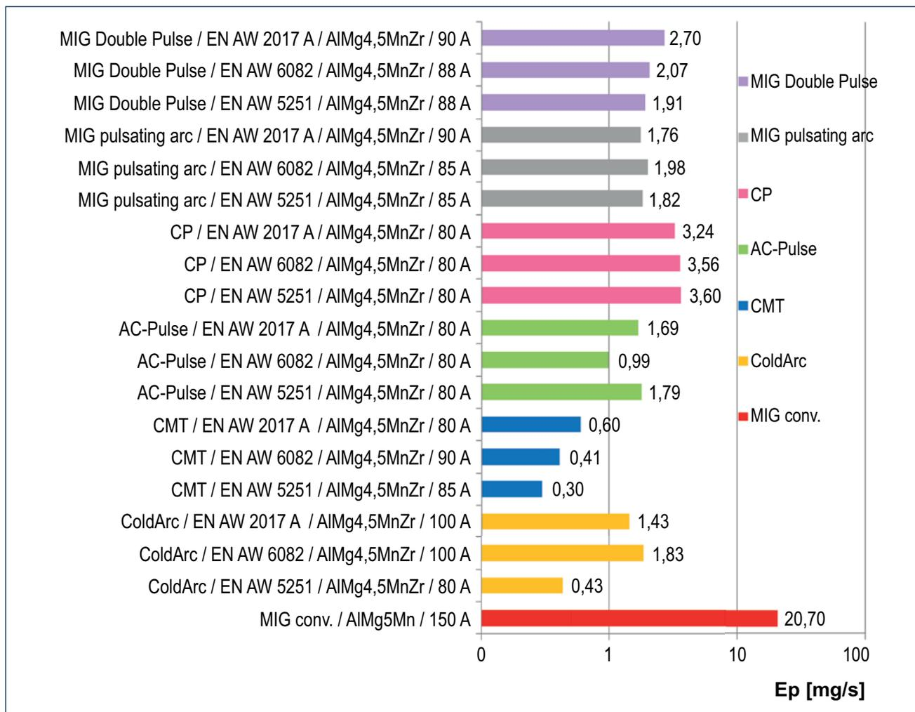
Fig. 31. Dust emission during welding of 5xxx, 6xxx and 2xxx series aluminium alloys with MIG welding and filler metal grade AlMg4.5MnZr
