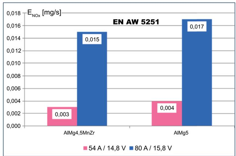
Fig. 12 NO<sub>x</sub> emission while welding aluminium alloy EN AW 5251 with Cold Process method using filler metal grades AlMg4.5MnZr and AlMg5Cr φ1.2 mm, in Ar-based shielding gas
