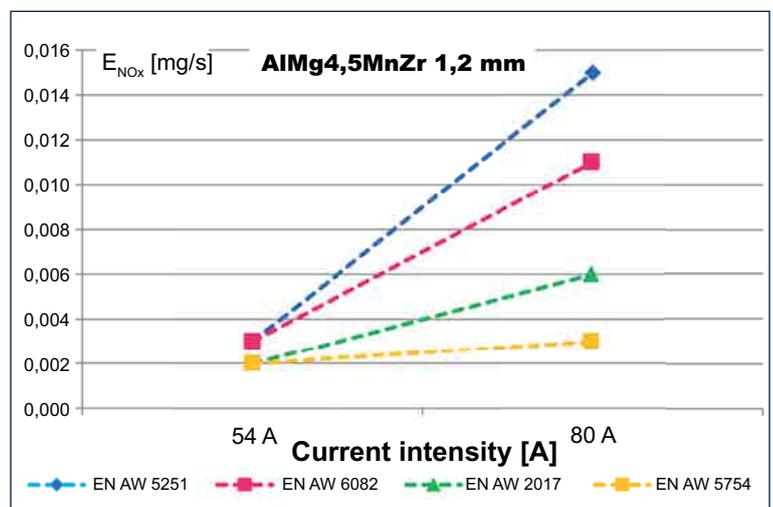
Fig. 14. Impact of current intensity on NO<sub>x</sub> emission while welding aluminium alloys of 5xxx, 6xxx and 2xxx series with Cold Process method using filler metal grade AlMg4.5MnZr φ1.2 mm, in Ar-based shielding gas
