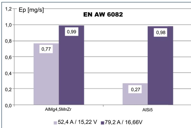
Fig. 17 Dust emission while welding aluminium alloy EN AW 6082 with AC Pulse method using filler metal grades AlMg4.5MnZr and AlSi5r  $\phi$ 1.2 mm, in Ar-based shielding gas
