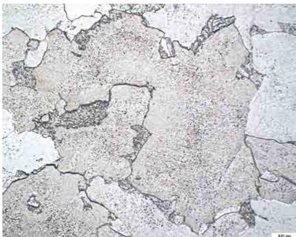
Fig. 10. SRCGHAZ area ( $T_{max} = 1250 + 700^{\circ}\text{C}$ ,  $t_{8/5} = 6$  s). Ferrite + pearlite. Hardness: 163.4 HV10
