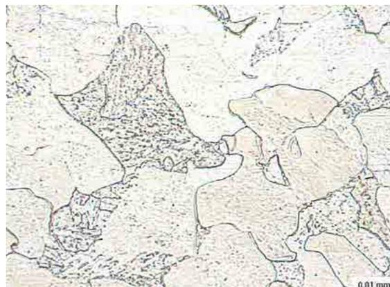
Fig. 6. Base metal of steel 13HMF after 132 782 hours' operation. Ferrite + bainite + fine dispersive carbides inside grains. Hardness: 212.4 HV10
