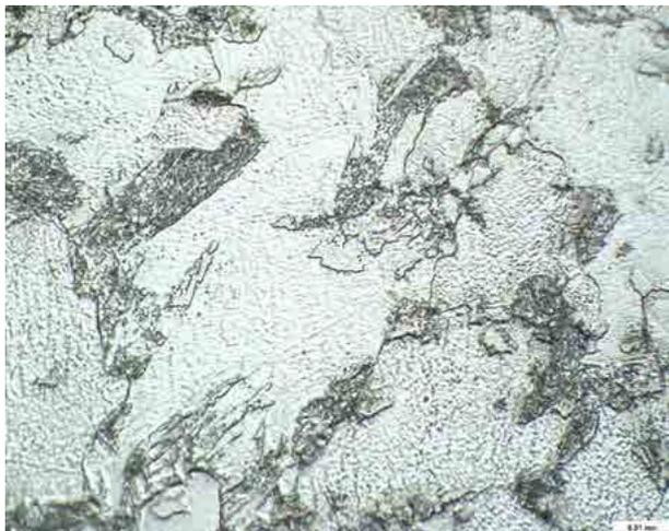
Fig. 9. ICCGHAZ area ( $T_{max} = 1250 + 800^{\circ}\text{C}$ ,  $t_{8/5} = 6$  s). Ferrite + pearlite. Hardness: 191.2 HV10
