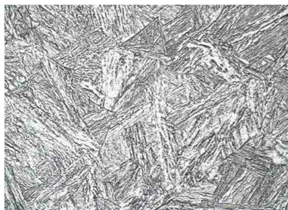
Fig. 7. CGHAZ area ( $T_{max} = 1250^{\circ}C$ ,  $t_{8/5} = 6$  s). Bainite + martensite. Hardness: 332.8 HV10
