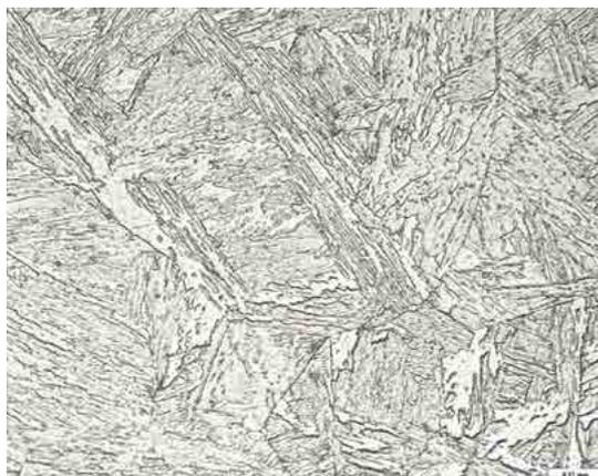
Fig. 11. HAZ area after tempering cycle ( $T_{max} = 1250 + 720 + 550^{\circ}\text{C}$ ,  $t_{8/5} = 6$  s). Bainite. Hardness: 321.2 HV10
