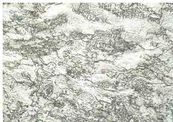
Fig. 8. FGHAZ area ( $T_{max} = 1250+950^{\circ}C$ ,  $t_{8/5} = 6$  s). Bainite + granular ferrite. Hardness: 264.8 HV10
