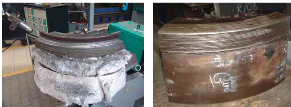
Fig. 3 Test element during (left) and after (right) overlay welding
