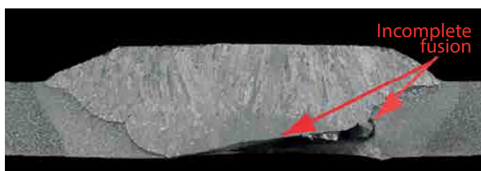
Fig. 5. Macrostructure of sample no. 2. Mag. 6.5x
