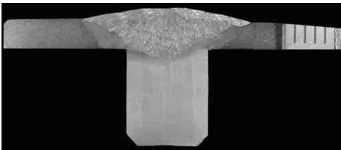
Fig. 17. Macrostructure of spot welded sample no. 19
