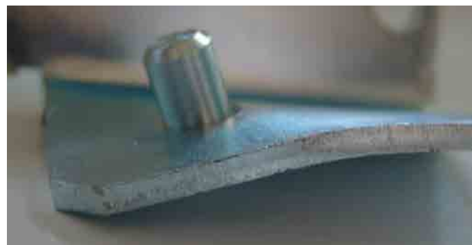
Fig. 4. Hinge element after workshop mechanical strength test; test result was positive
