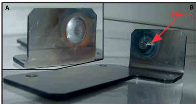
Fig. 2. Element of hinge directly after welding: A – view from plug weld face, B – view from pin (visible notch)
