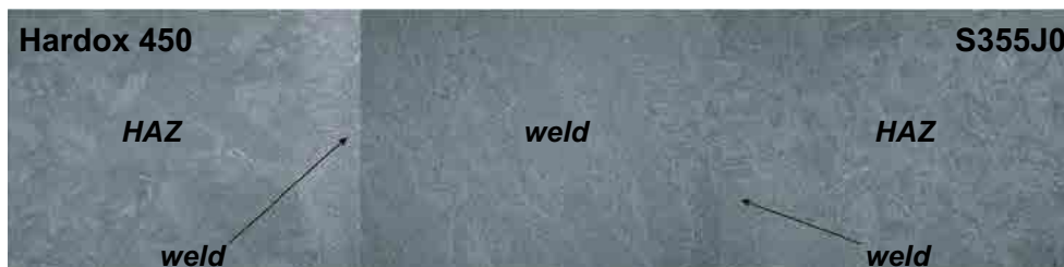
Fig. 6. Microstructure of MMA-welded joint (111); mag. x200, etchant Mi1Fe
