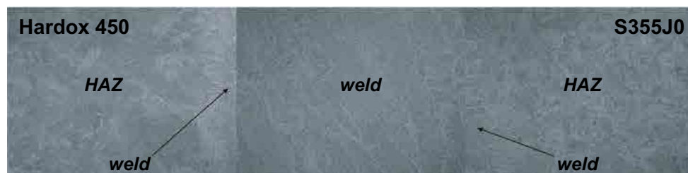
Fig. 7. Microstructure of MAG-welded joint (135); mag. x200, etchant Mi1Fe
