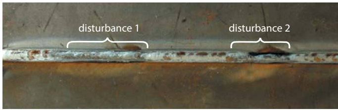
Fig. 5. View of welded joint made after introducing disturbance in the form of filler metal placed in weld groove
