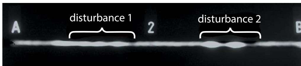
Fig. 13. Radiogram of MAG welded joint after introducing disturbance in the form of filler metal
