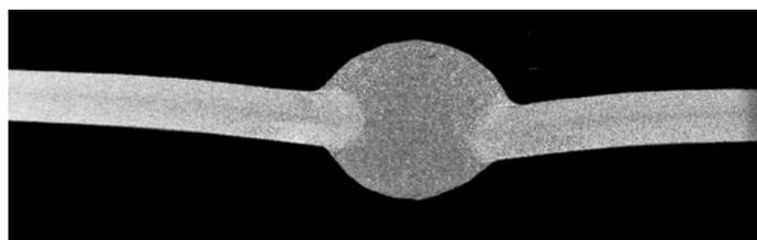
Fig. 5. Macrostructure of CMT welded joint made of 2.0 mm thick EN AW 6082 alloy after heat treatment, filler metal AlMg4.5MnZr  $\phi$ 1.2 mm, mag. 5x
