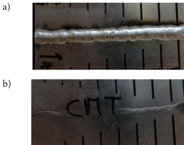
Fig. 3. Result of Houldcroft test carried out with CMT method a) face; b) root
