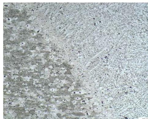
Fig. 7. Microstructure of CMT welded joint made of 2.0 mm thick EN AW 6082 alloy after heat treatment, HAZ view (on the right - base metal, on the left - weld), filler metal AlMg4.5MnZr  $\phi$ 1.2 mm, etching with Keller's reagent, mag. 100x
