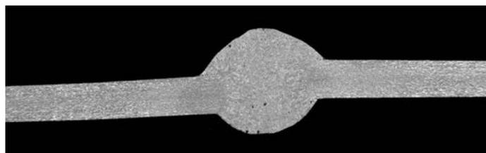
Fig. 4. Macrostructure of CMT welded joint made of 2.0 mm thick EN AW 6082 alloy, filler metal AlMg4.5MnZr  $\phi$ 1.2 mm, mag. 5x
