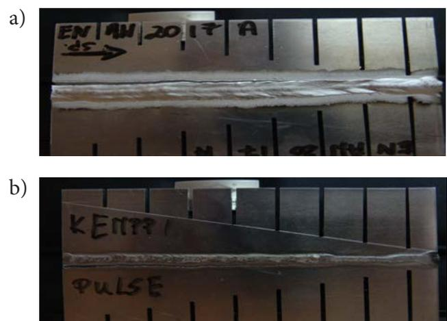
Fig. 2. Result of Houldcroft test carried out with MIG-Pulse method a) face; b) root
