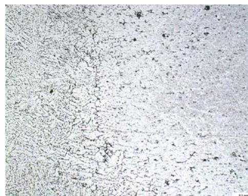
Fig. 6. Microstructure of CMT welded joint made of 2.0 mm thick EN AW 6082 alloy, HAZ view (on the right - base metal, on the left - weld), filler metal AlMg4.5MnZr  $\phi$ 1.2 mm, etching with Keller's reagent, mag. 100x
