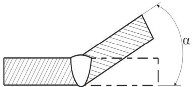
Fig. 1. Joint angular deformation
