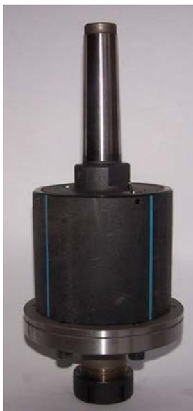
Fig. 4. Measuring head of FSW Weld Monitor system
