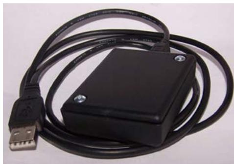
Fig. 5. Receiver module
