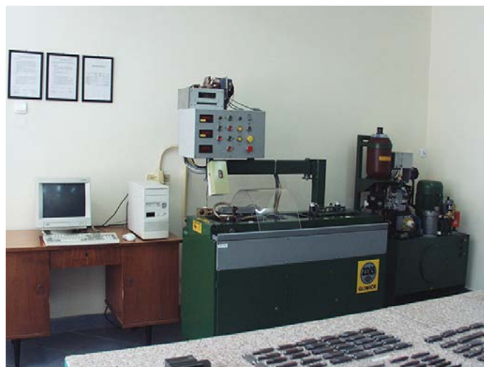
Fig. 4. Main view of the simulator of thermal-strain cycles produced by Instytut Spawalnictwa (version from 1996)
