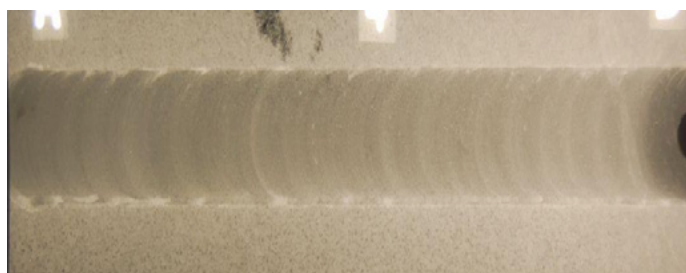
Fig. 3. Radiogram of the joint made of casting aluminium alloy EN AC-43200. Welding parameters: V_n = 1300 \text{ rev./min} , V_z = 200 \text{ mm/min}
