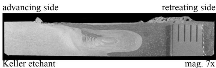
Fig. 11. Macrostructure of FSW weld made of EN AW- 2017A (on the advancing side) and EN AC-43200 (on the retreating side) alloys, built up with a conventional tool. Welding parameters: V_n=560 rev./min, V_z=112 mm/min
