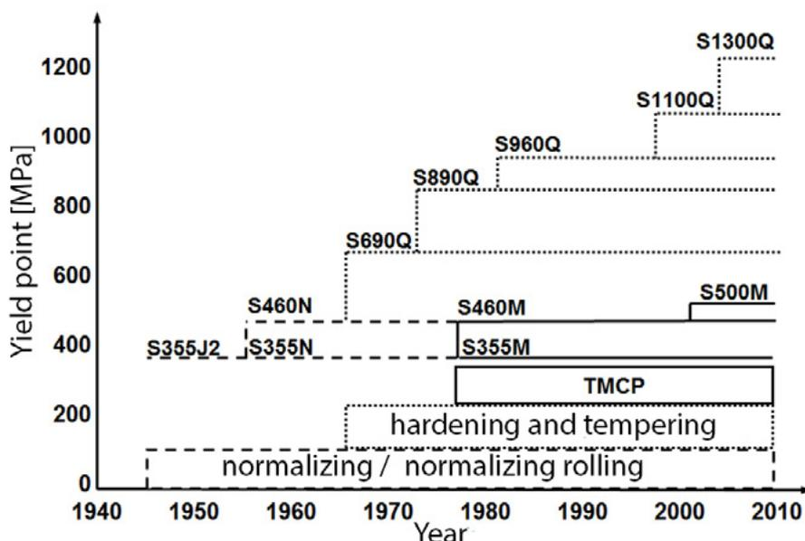
Fig. 1. Development of structural steels (TMCP – Thermo-Mechanical-Control-Process – process of thermo-mechanical rolling) [1]
