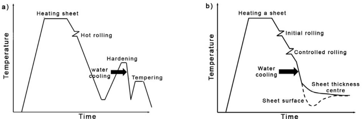
Fig. 4. Diagrams of production processes of toughened steels a) hardening and tempering processes, b) direct hardening process.
