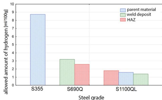
Fig. 10. Allowed hydrogen content in parent metal depending on steel grade (yield point) [44]
