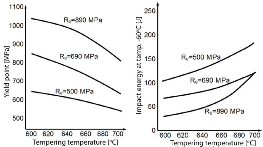
Fig. 3. Impact of tempering temperature on yield point a) and impact strength b) of three toughened steels [13]
