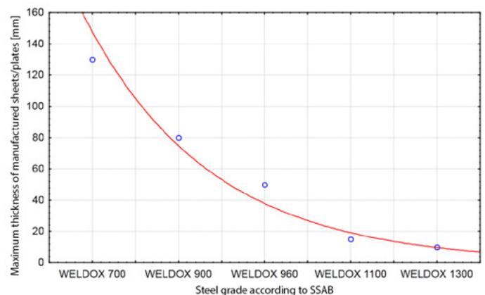
Fig. 6. Maximum thickness of standard sheets made of steel Weldox, other thicknesses available on the basis of individual orders [24-28]
