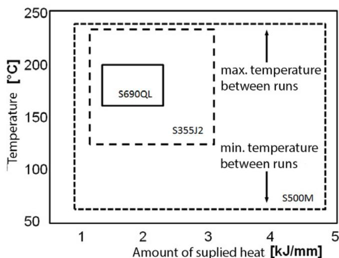
Fig. 9. Typical welding conditions for structural steels (S355J2 – 80 mm, S500M – 50 mm, S690QL – 30 mm) [1]
