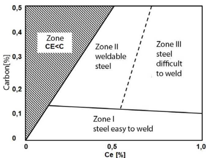
Fig. 7. Impact of carbon content and carbon equivalent CE on structural weldability : I – zone free from susceptibility to cracking, II – zone with susceptibility to cracking depending on welding conditions, III – zone of high susceptibility to cracking independent of welding conditions [29]
