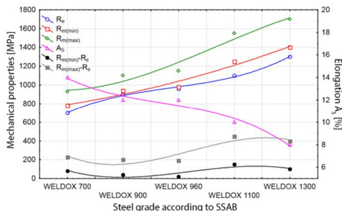
Fig. 5. Mechanical properties of steel Weldox [18-22]
