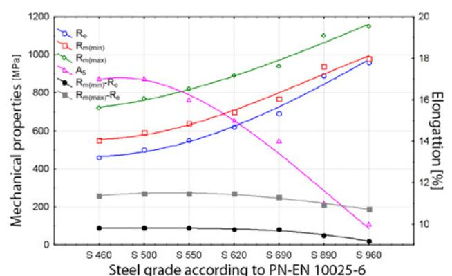
Fig. 8. Mechanical properties of toughened steels [4]
