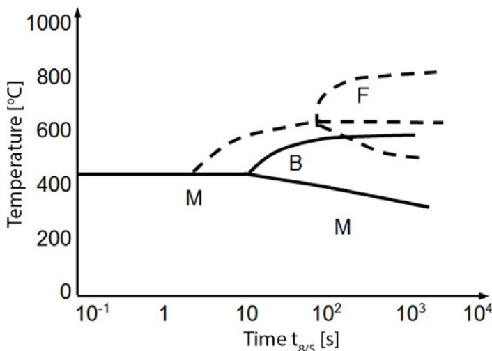
Fig. 2. CCT diagram for welding conditions showing the impact of boron micro-addition on the curves of the beginning of cooled austenite transformations in of Mn-Cr-Mo-Ti steel in the function of time  $t_{8/5}$ : - - steel without boron, — steel with boron, (0.17% C; 0.85% Mn; 0.005% N; 0.30% Cr; 0.85% Mo; 0.03% Ti; 0.0016%) B [14]
