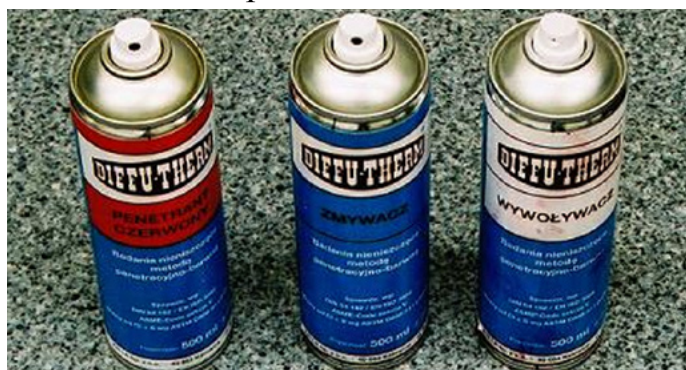
Fig. 3. Set of aerosols “Diffu - Therm” used in the liquid-penetrant inspection of plates with discontinuities
