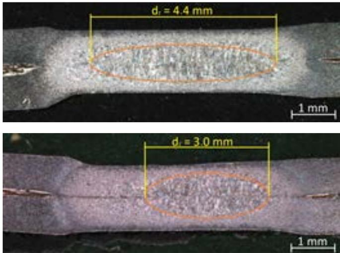
Fig. 4. Results of metallographic tests concerning steel DC 01 and a) welding current of 9.2 kA and b) welding current of 8.4 kA
