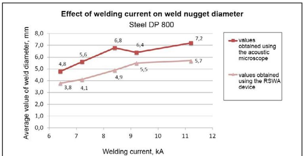
Fig. 9. Effect of welding current used for the welding of steel DP 800 on the size of the spot weld nugget diameter measured using scanning acoustic microscopy and the RSWA device
