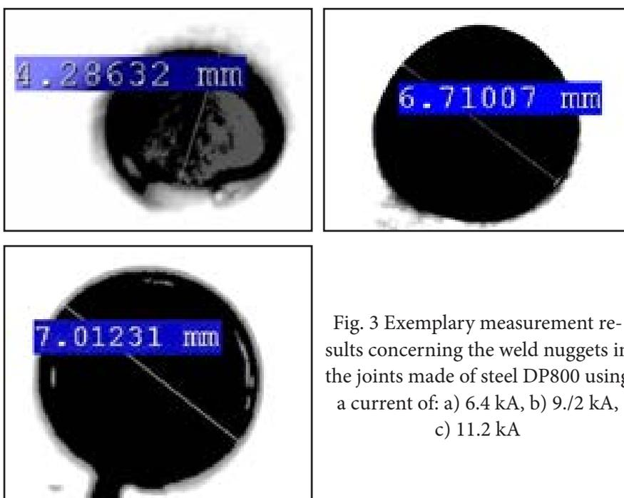
Fig. 3 Exemplary measurement results concerning the weld nuggets in the joints made of steel DP800 using a current of: a) 6.4 kA, b) 9./2 kA, c) 11.2 kA
