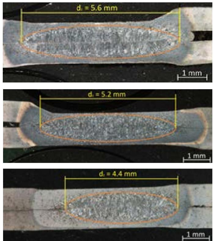
Fig. 6. Results of metallographic tests concerning steel DP900 and a) welding current of 9.2 kA, b) welding current of 8.4 kA and c) welding current of 7.2 kA
