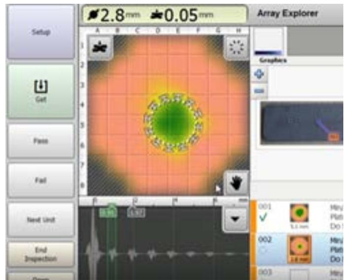
Fig. 2. User interface and the manner of a weld nugget diameter measurement using the RSWA device [10]
