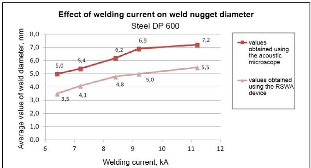
Fig. 8. Effect of welding current used for the welding of steel DP 600 on the size of the spot weld nugget diameter measured using scanning acoustic microscopy and the RSWA device
