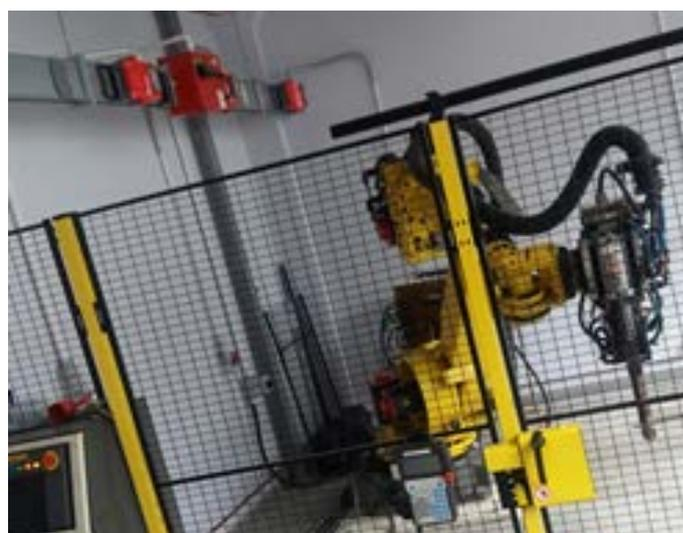
Fig. 1. Robotic welding station used in the welding process
