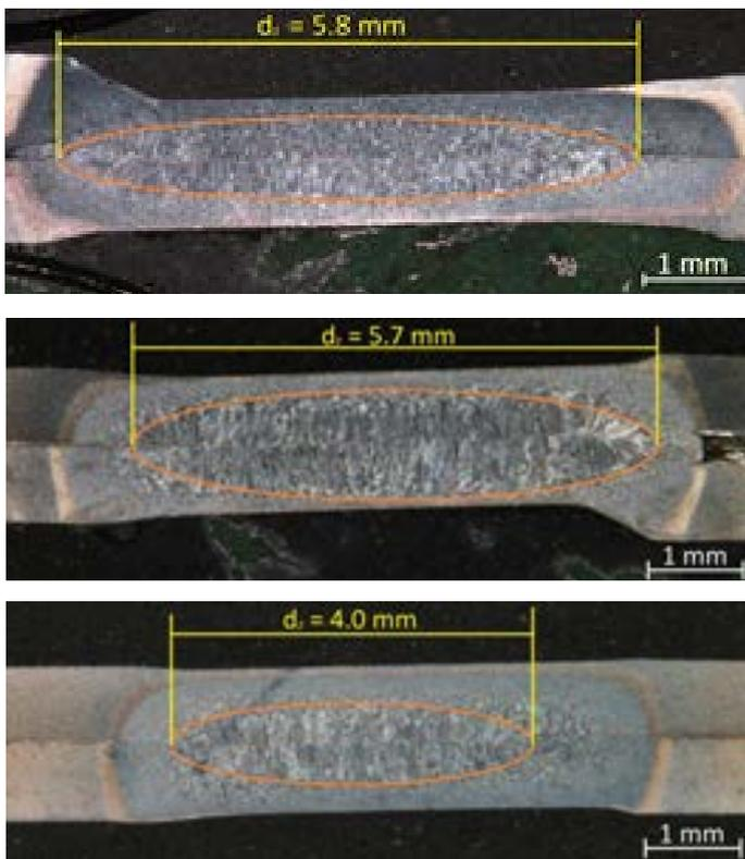
Fig. 5. Results of metallographic tests concerning steel DP600 and a) welding current of 9.2 kA, b) welding current of 8.4 kA and c) welding current of 7.2 kA
