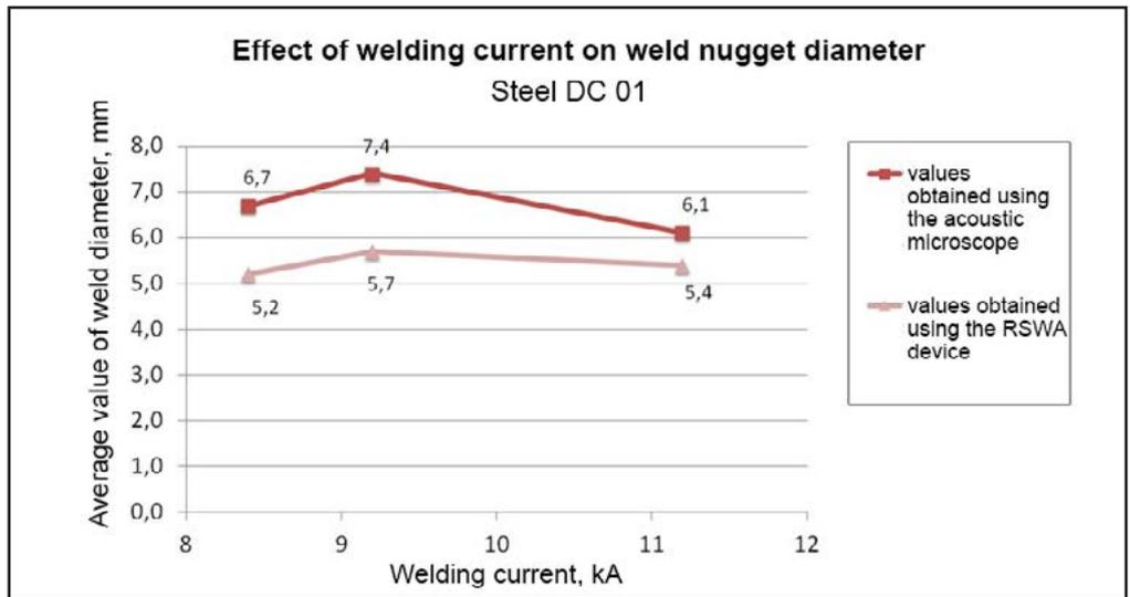
Fig. 7. Effect of welding current used for the welding of steel DC 01 on the size of the spot weld nugget diameter measured using scanning acoustic microscopy and the RSWA device
