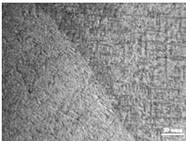
Fig. 12. Microstructure the welded joint made of alloy VT22, subjected to annealing
