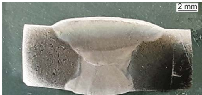
Fig. 2. Macrostructure of the test joint
