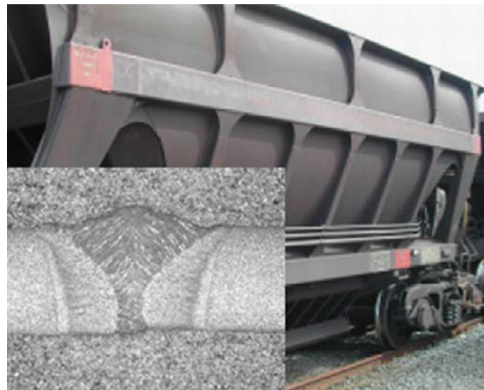
Fig. 5. Hybrid welding of carriage elements; high strength steel; CO 2 laser having a power of 20 kW [19]
