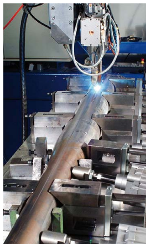
Fig. 3. Welding of tubular support performed using the HLAW method [26]
