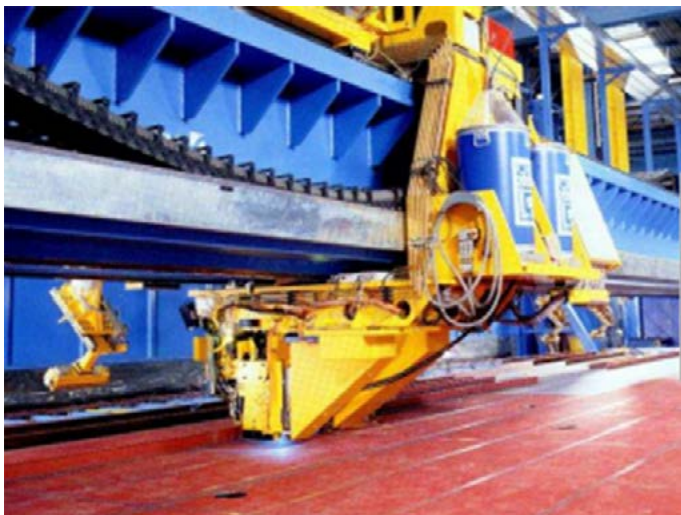
Fig. 4. Hybrid welding of ship plating panels, butt joints and the welding of stiffening elements. Laser CO 2 12 kW. Meyer Werf Shipyard, Germany [22]
