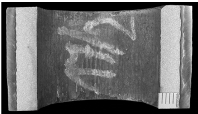
Fig. 2. Macrostructure of the tube ( \varnothing 44.5 \times 5.0 ) mm made of steel 13CrMo4-5 with the two-layer overlay weld made of nickel alloy Inconel 625
