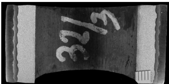
Fig. 3. Macrostructure of the tube ( \varnothing 44.5 \times 5.0 ) mm made of steel 13CrMo4-5 with the three-layer overlay weld made of nickel alloy Inconel 625
