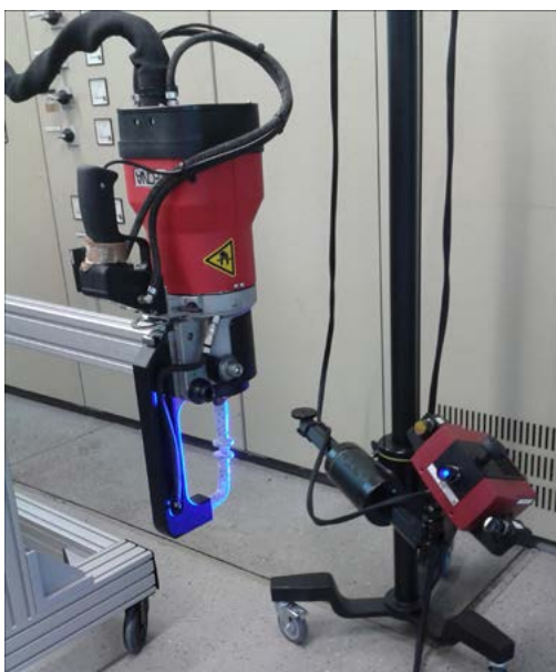
Fig. 7. Repair welding gun including bracket and optical measuring equipment
