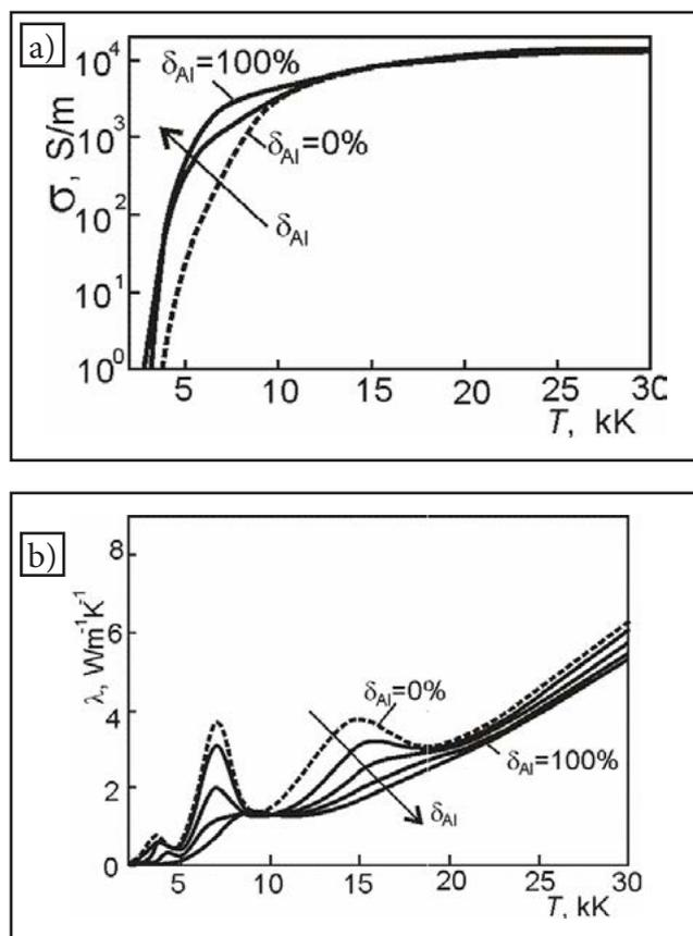
Fig. 1. Selected physical characteristics of mixtures of gases and metal vapours under a pressure of 1 bar
