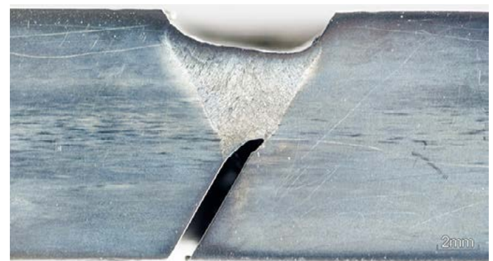
Fig. 6. Cross-section of the joint welded in air: specimen P1, q_{el} = 0.87 kJ/mm; the lack of welding imperfections; etchant: Beraha
