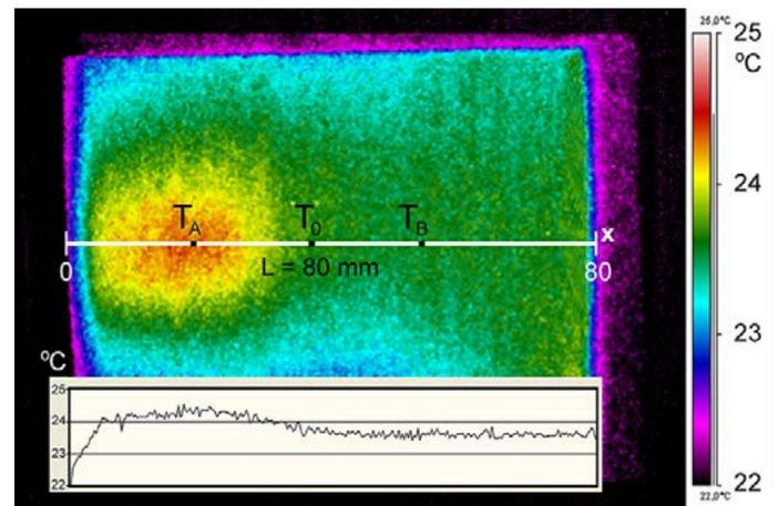
Fig. 5. Thermographic image of the surface of specimen 2 with the momentary temperature profile along the straight line representing the location of the adhesive layer axis
